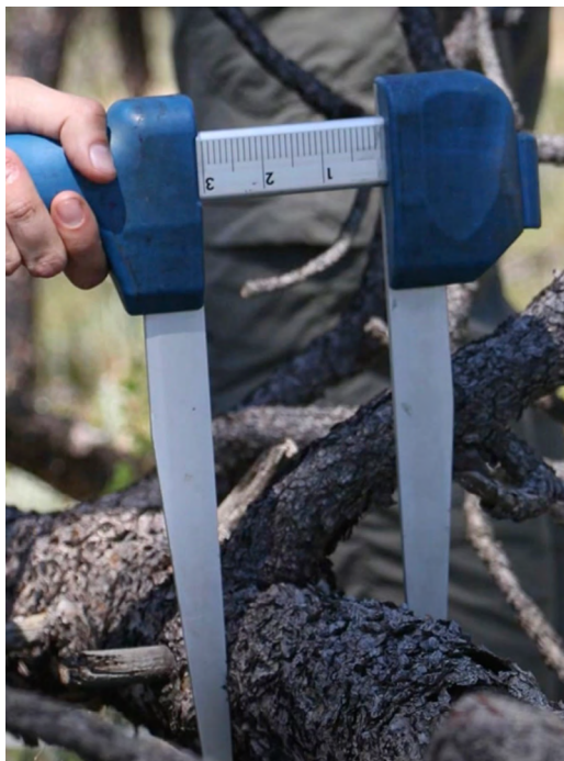
Measuring the diameter of a coarse woody fuel on a transect.
