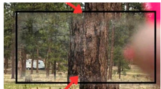
Variable radius plots use a wedge prism to determine which trees are "in" the plot.
