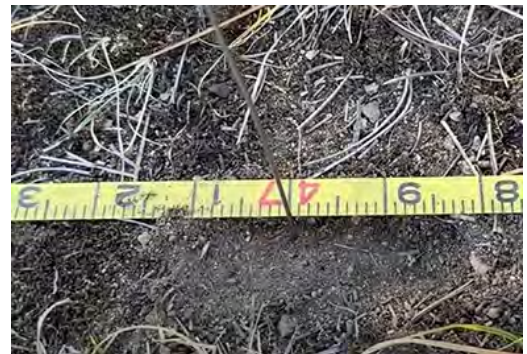
Using a pin flag to record each substrate encountered at set points along a transect.
