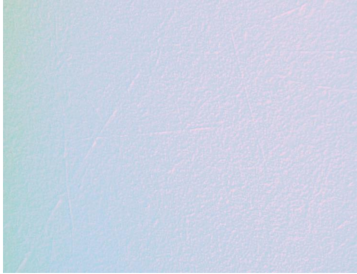
Figure 4.7: Surface image of \text{TiO}_2\text{:GeO}_2\text{:ZrO}_2 after annealing to 800C. Roughened surface is visible.
