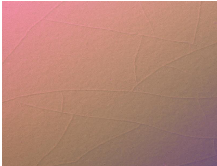
Figure 4.6: Surface image of \text{TiO}_2:\text{SiO}_2:\text{ZrO}_2 after annealing to 700C. Cracking is visible.
