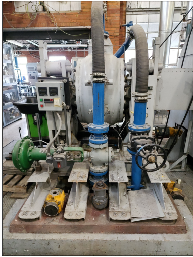
Figure 2.7: The GMV's load is controlled using a water-brake dynamometer.
