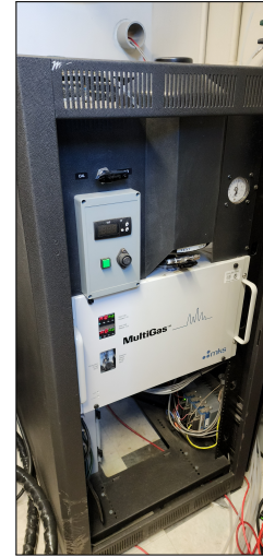
Figure 2.8: The MKS FTIR used to determine engine out emissions.
