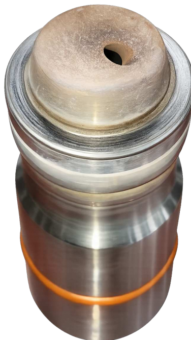
Figure 2.6: The Cooper Bessemer OEM single nozzle pre-combustion chamber.
