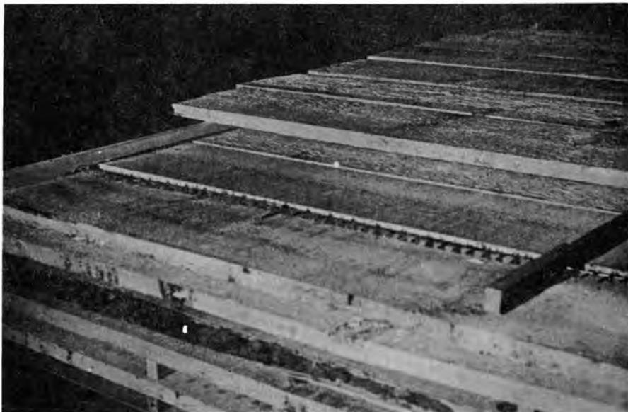
FIGURE 7 : DELTA WING VORTEX GENERATORS
