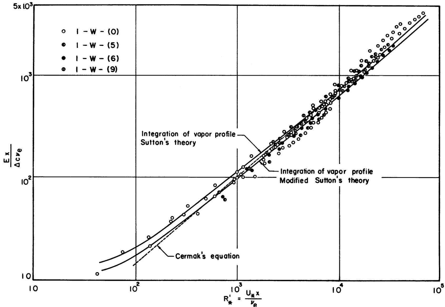
FIGURE 3 VARIATION OF  $N$  WITH  $R'_*$  FOR TURBULENT BOUNDARY LAYER (BUFFERS WET, ALL DATA)
