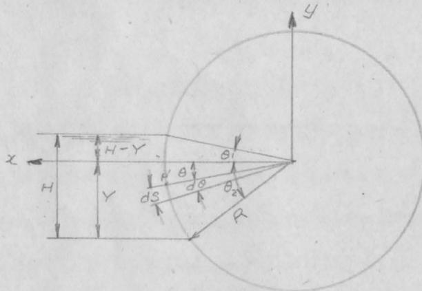
Let  $ds$  = any infinitesimal segment of arc along the face of gate
