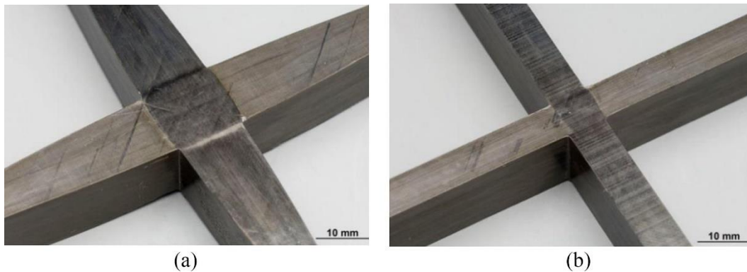
Figure 5: Methods for reducing intersection buildup. (a) Widening of the stiffeners by spreading the tows. (b) Alternating discontinuous tows [14].
