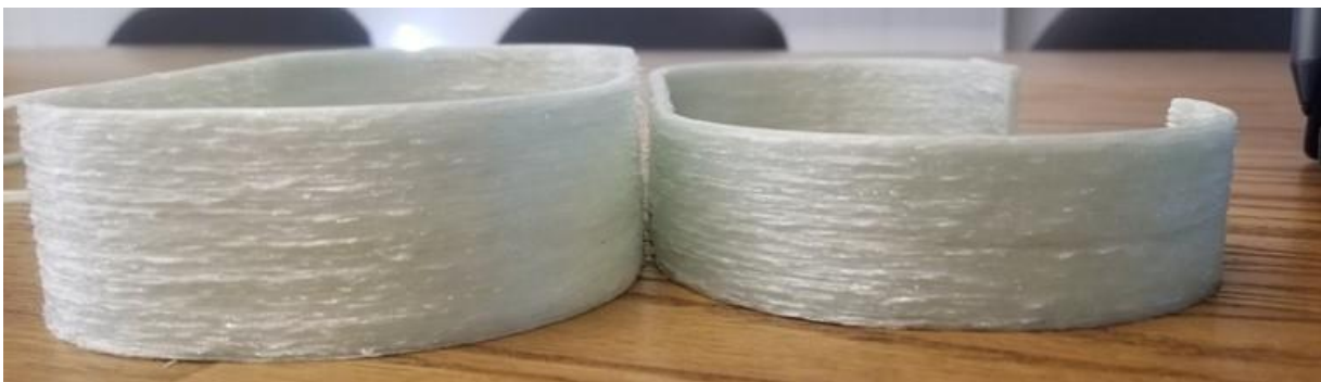
Figure 14: Comparison of final height of 0.5 mm layer height (left) and 0.4 mm layer height (right) loop print samples.
