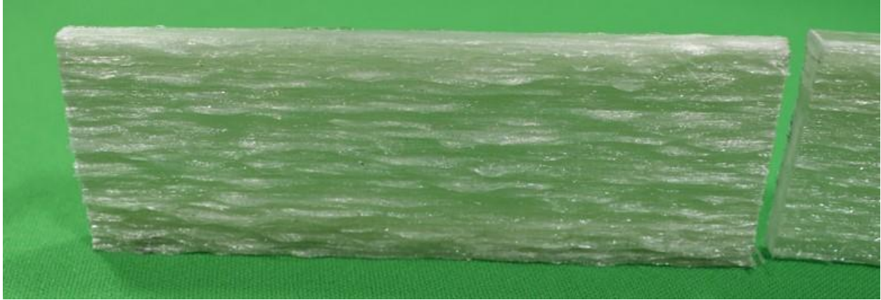
Figure 18: Close-up image of the as-printed rough texture of the walls of the stiffener rib samples.
