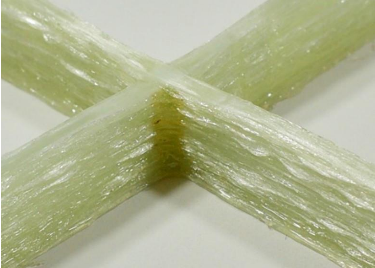
Figure 61: Close-up of intersection node of the stiffener grid intersection point sample.
