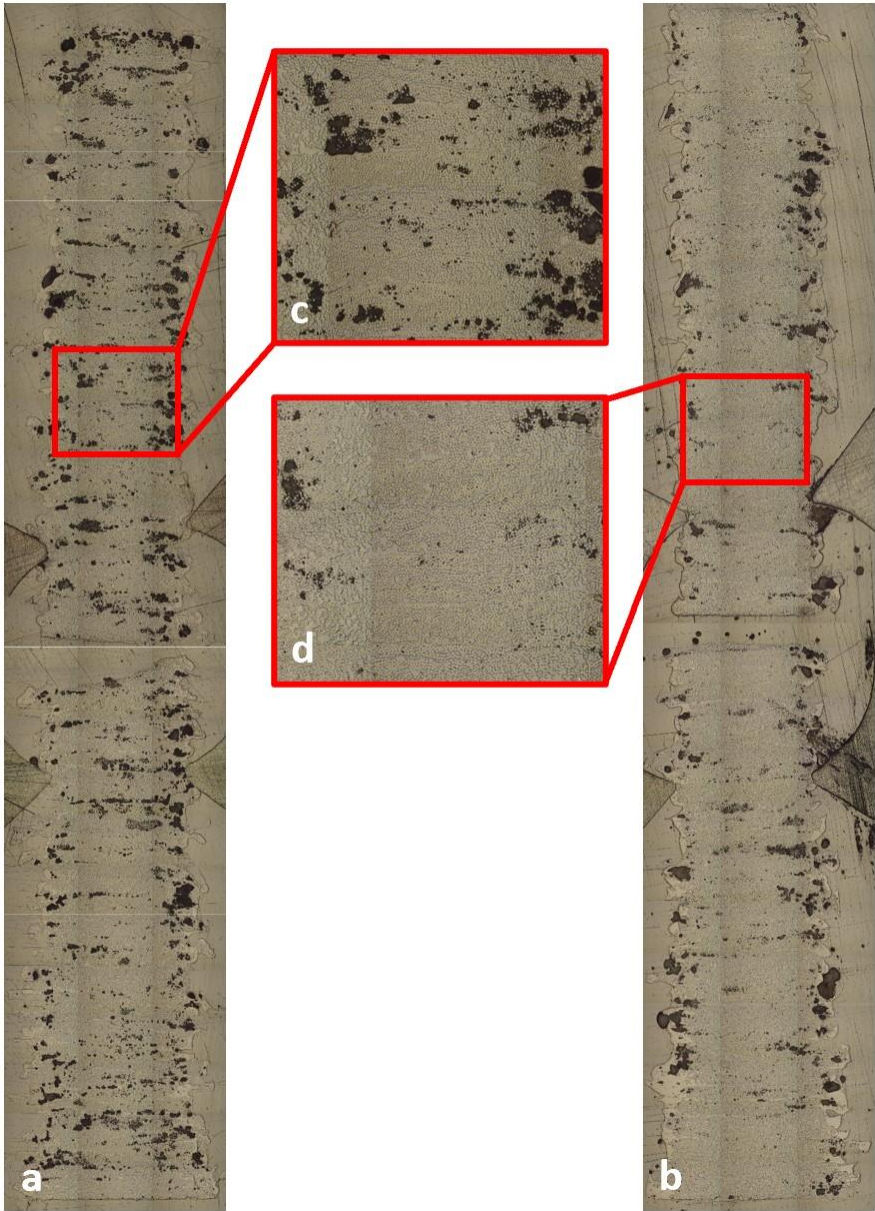
Figure 45: (a) Micrograph of force measured S specimen. (b) Micrograph of force measured E specimen. (c) Zoomed in portion of S specimen micrograph. (d) Zoomed in portion of E specimen micrograph.
