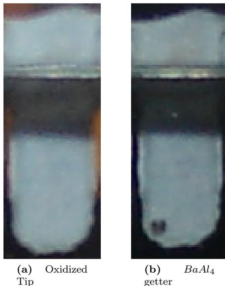
**Figure 5.9:** Photograph(a) is a picture of the oxidized barium metal tip before any ablation shots. Photograph(b) shows the tip after the first current signals was detected.
