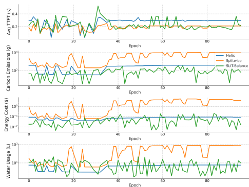
Figure 5: Per-epoch metric comparison for LLM scheduling across the Helix , Splitwise , and SLIT frameworks.
