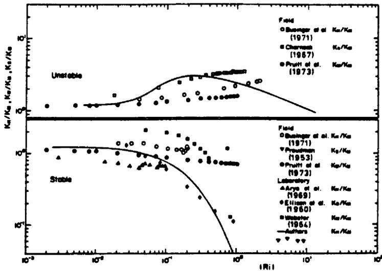
Fig. 4.4. Comparison of the Ueda's *et al.*, (1981) (line labeled Authors) results on  $K_H/K_M$  with those of other investigators. [From Ueda *et al.*, (1981)].
