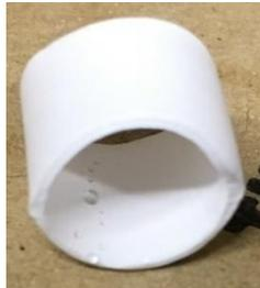
*Figure 2.7: ePTFE graft that was spray coated with NaHA/DiH<sub>2</sub>O. The water can be seen beading up on the inner lumen of ePTFE because of water high surface tension, and that prevents the liquid from wetting and soaking into ePTFE.*
