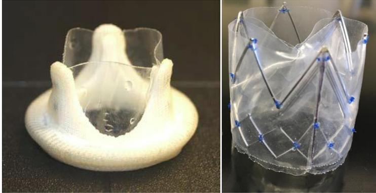
*Figure 1.6: HA treated surgical (left) and transcatheter (right) heart valves containing flexible leaflets made from LLDPE [74].*
