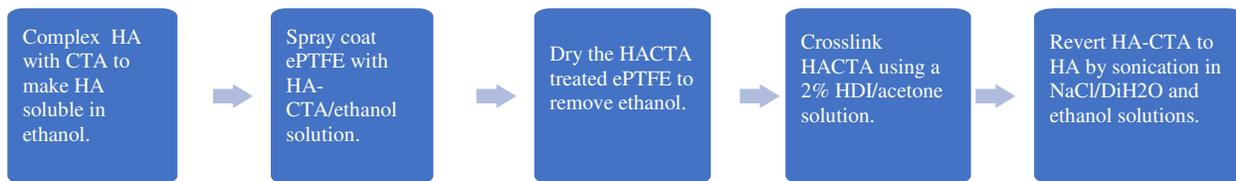
Figure 2.8: Schematic of the HA-ePTFE fabrication process.
