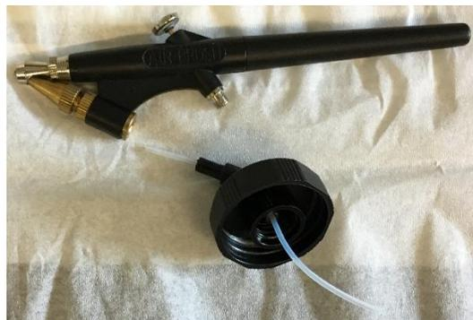
Figure 2.4: Image of the airbrush used for the HA treatment.
