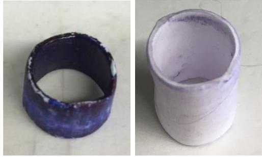
*Figure 2.17: Pictures of HA-ePTFE (left) and ePTFE (right) after stained with TBO. It is evident that the treatment creates a confluent layer of HA on the inner lumen of ePTFE graft.*
