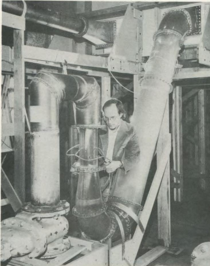
HYDRAULIC SURGE--Thrust along by the unseen pressure exerted by a difference in elevation, or "head," water surges through this plexiglass suction tube under the eyes of hydraulic engineer Perry L. Johnson at the Bureau of Reclamation's engineering laboratories in Denver. Johnson is directing research into the design and operation of the Lake Havasu Pumping Plant, a principal feature of the Central Arizona Project.
