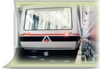
As noted in the above picture the rope propulsion is provided at one side of the vehicle. This was not the first application of the Otis rope-propelled, air-supported technology in North America since they had installed, in 1985, a dual lane shuttle system between Harbor Island and downtown Tampa, Florida. The system is no longer in operation.
