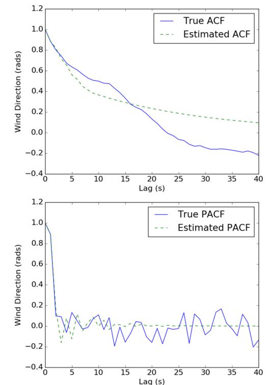
Statistical characteristics plotted of wake displacement with ACF on top and PACF on bottom.
