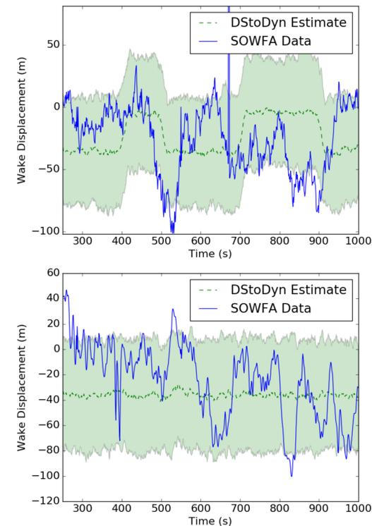
Time series plots of wake displacement with turbine 0 on top and turbine 1 on bottom showing two standard deviations.
