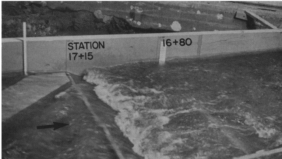
Figure 5 - Flow Conditions In Vicinity Of Drop Structure At A Discharge Of 2702 cfs.
