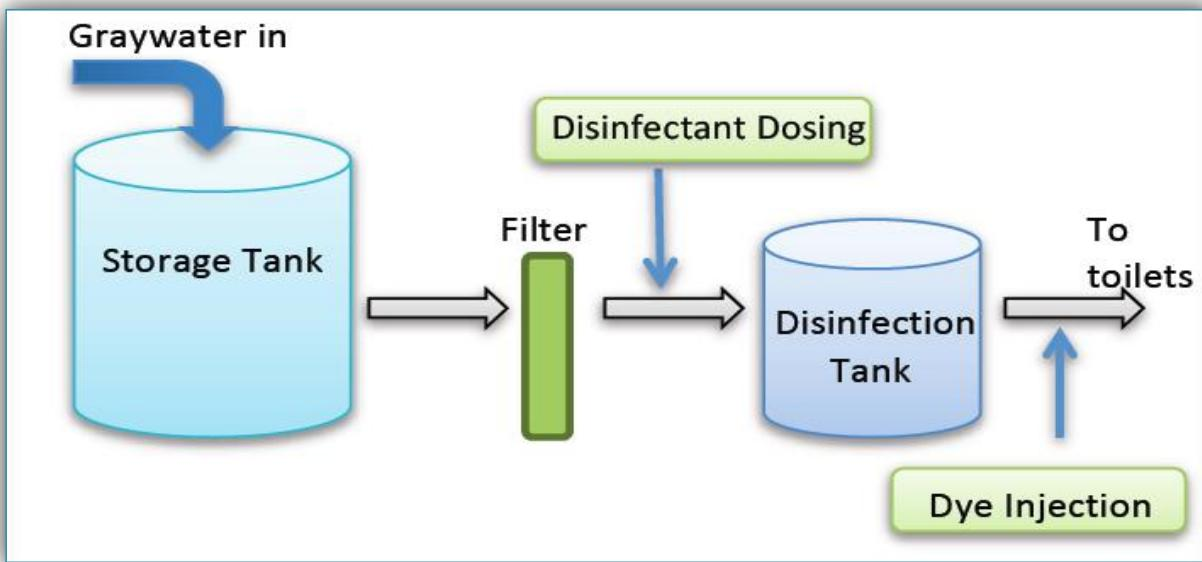
Figure 2: Graywater Treatment System Schematic
