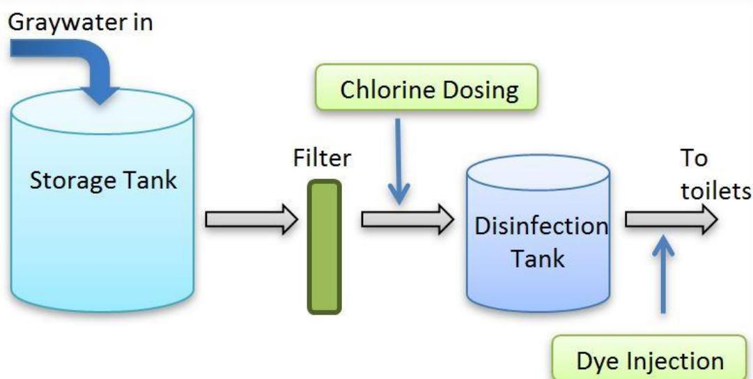
**Figure 6.1 Graywater Treatment Process Schematic**
