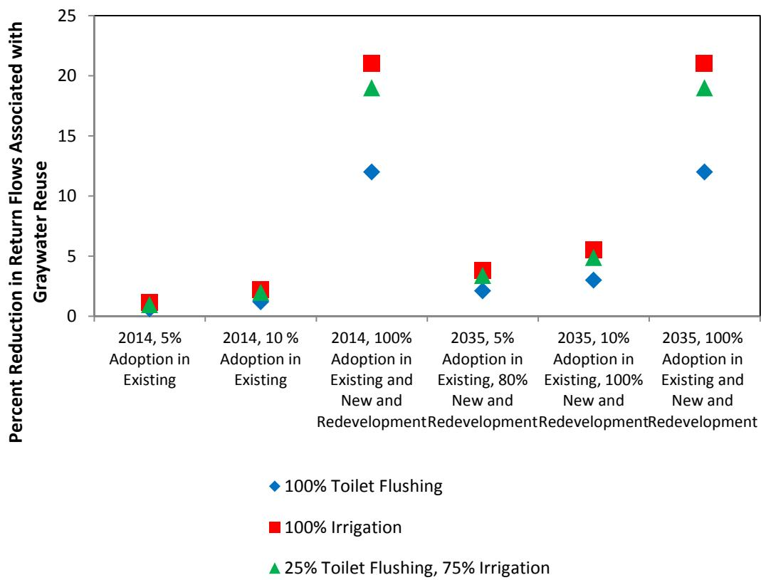
**Figure 4.11 Percent Reduction in Return Flows Associated with Graywater Reuse in Fort Collins, Colorado for Scenarios 1, 2, and 3 in 2014 and 2035**
