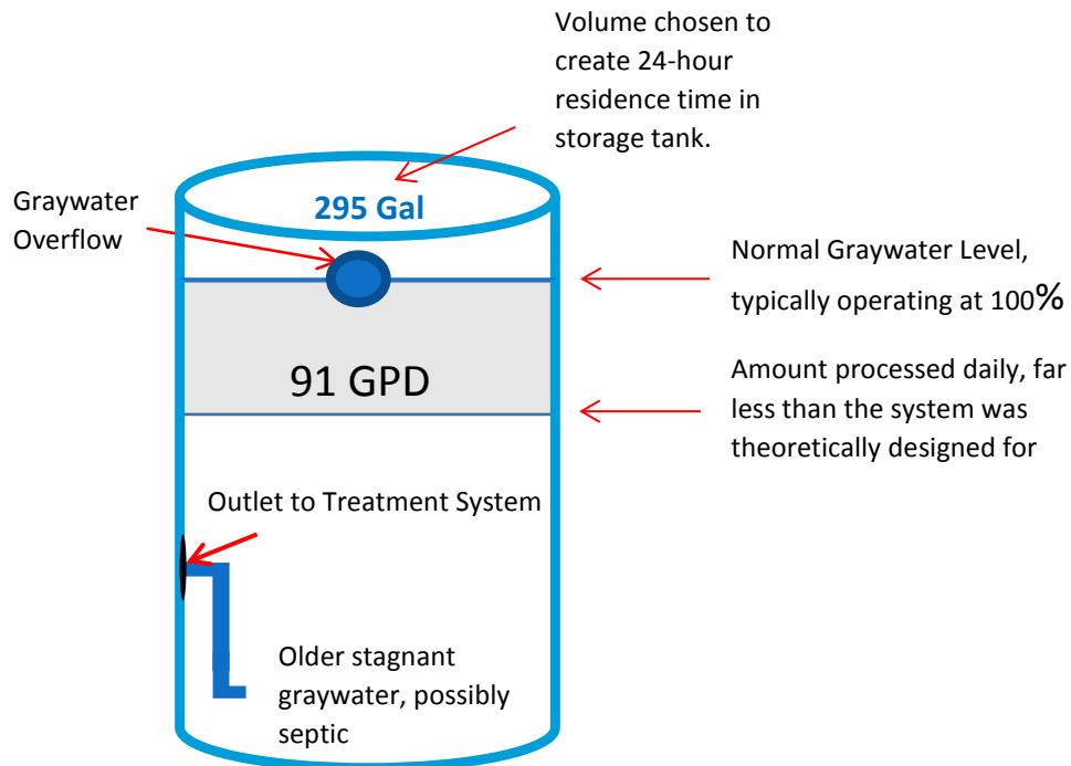
Figure 6.6 Schematic of Graywater Storage Tank Concerns
