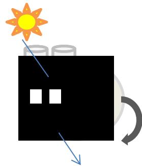
7. Read the result in mg/L and record on the form given to you. If the best match occurs between two color segments, determine the value halfway between the two printed numbers.
