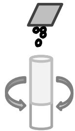
5. Insert the second tube into the right opening of the comparator.
