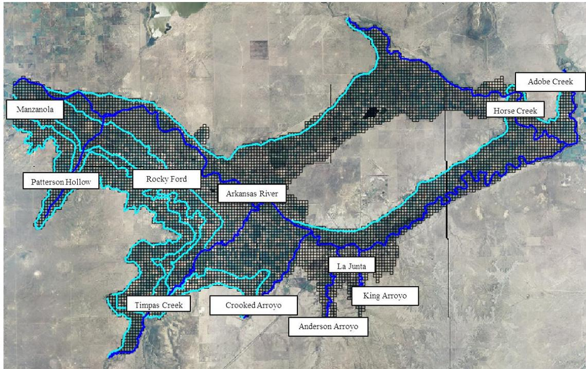
Figure 2.2. MODFLOW-UZF model cell discretization within the LARV.
