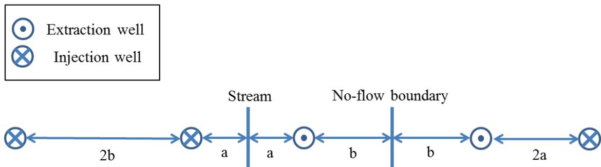
Figure 2.3. Image well scheme applied to the Glover-Balmer solution to account for a no-flow boundary.
