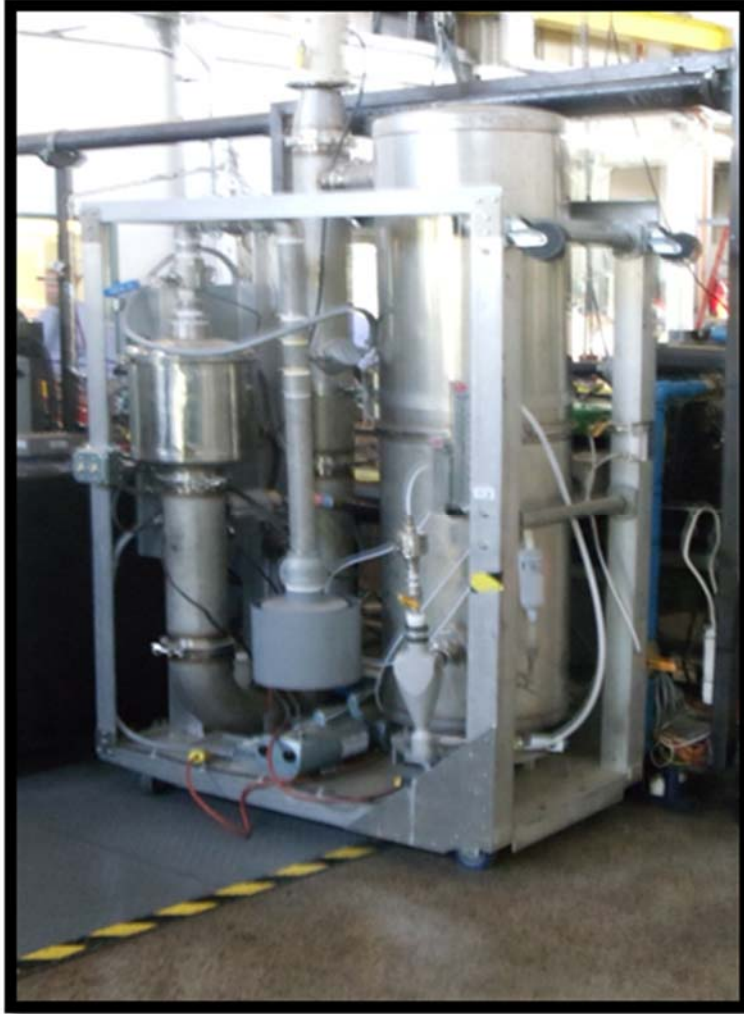
Figure 6: Actual Dilution Tunnel Set UP
