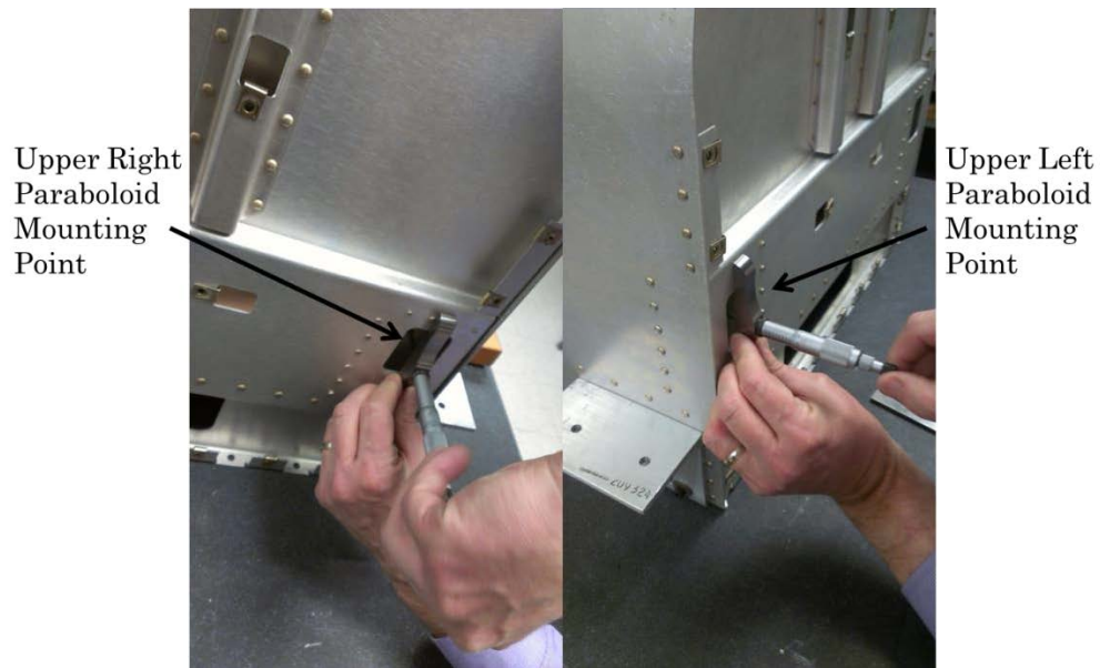
Figure 30: Depth Micrometer Measurements Used to Characterize Offset of Upper Paraboloid Mounting Points.
