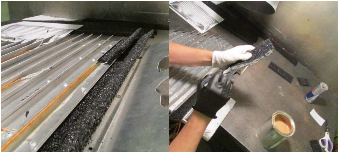
Figure 89: Process of Gluing Eccosorb to Target (1/2)
