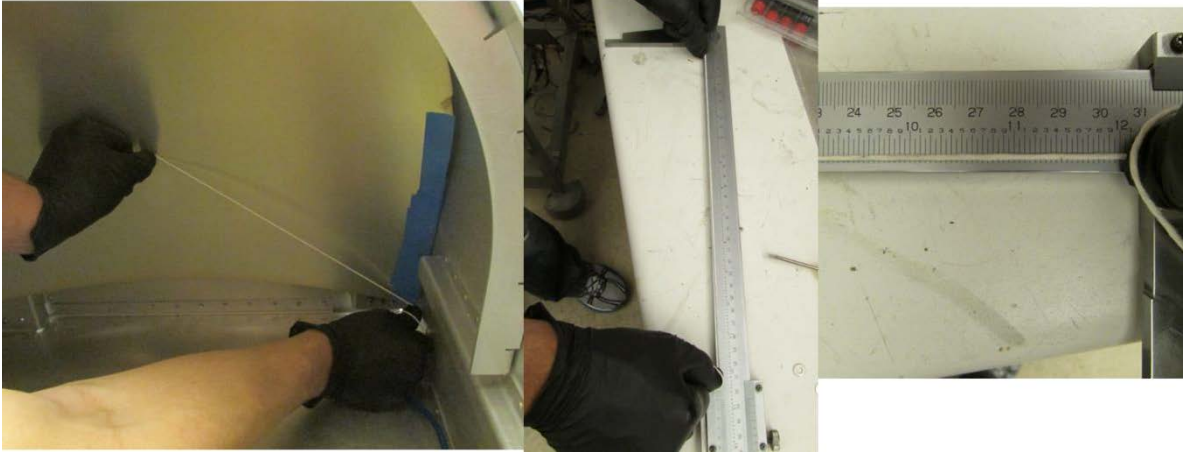
Figure 55: Illustration of Measurement Technique Used to Determine the Distance Between the Laser Illumination Point and each Corner of the Offset Paraboloid.
