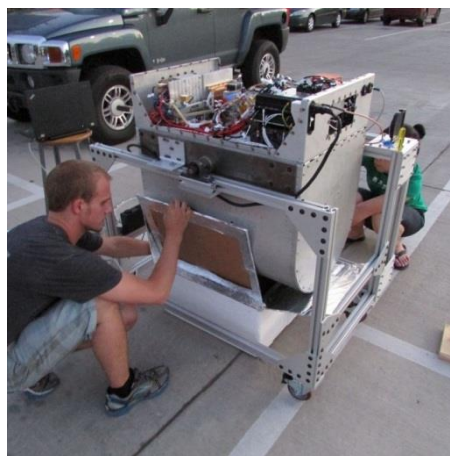
Figure 150: HAMMR Viewing the Styrofoam LN2 Calibration Target with Cardboard Flaps in Use
