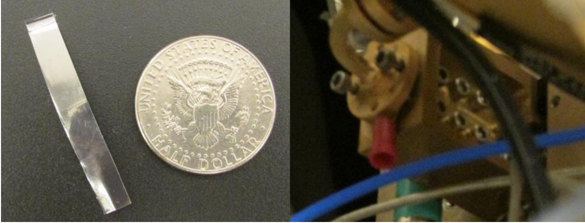
Figure 137: Antistatic Bag Attenuator across the Diplexer Waveguide Output
