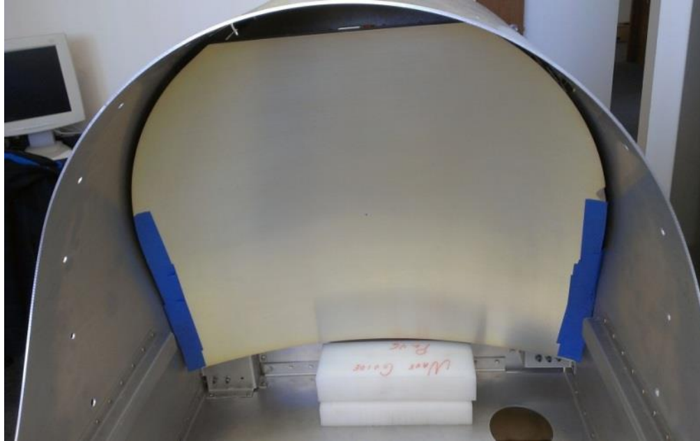
Figure 29: Offset Paraboloid Integrated in HAMMR Chassis.
