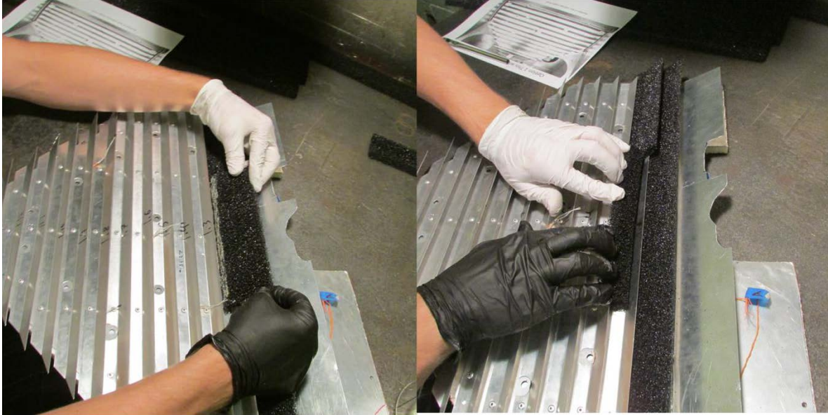
Figure 90: Process of Gluing Eccosorb to Target (2/2)
