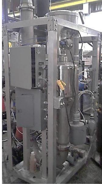
Figure 3.6: Particulate matters dilution tunnel
