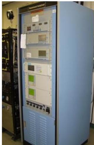
Figure 3.3: Rosemount 5-Gas analyzer rack with Siemens analyzers
