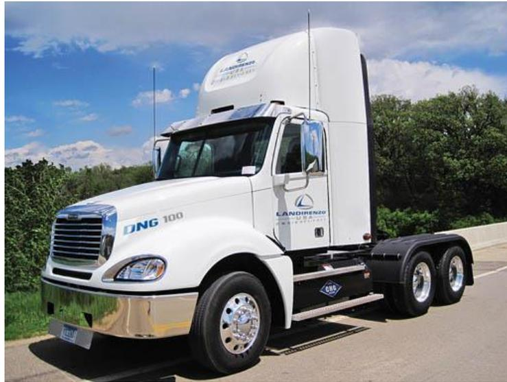
Figure 1.9: A diesel truck running on CNG and diesel. Conversion kit by Landi Renzo
