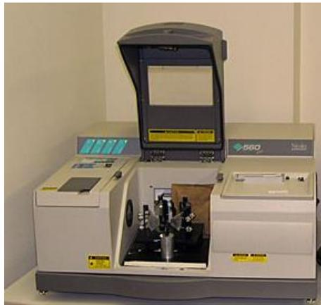
Figure 3.4: Nicolet Magna 560 FTIR spectrometer used in the research
