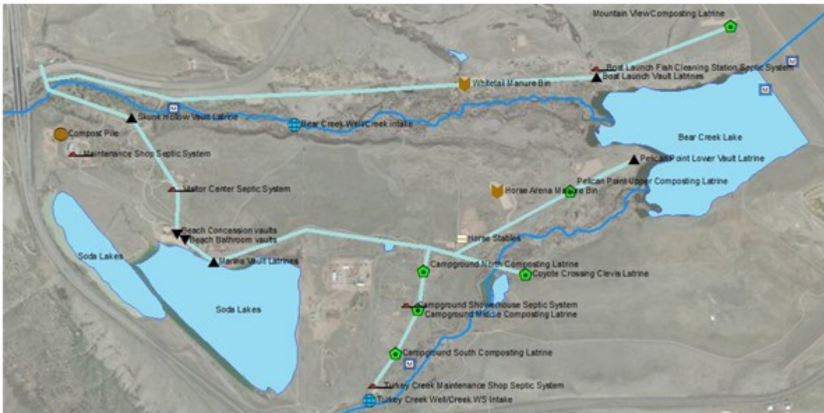
Figure 3. Approximately six miles of sewer line would be required to connect BCLP to Morrison WWT
