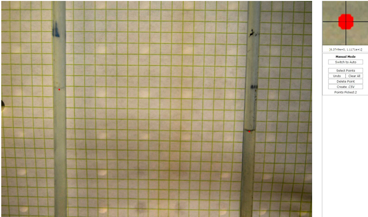
Figure 32: Manometer readings of pressure drop and markers of height difference.
