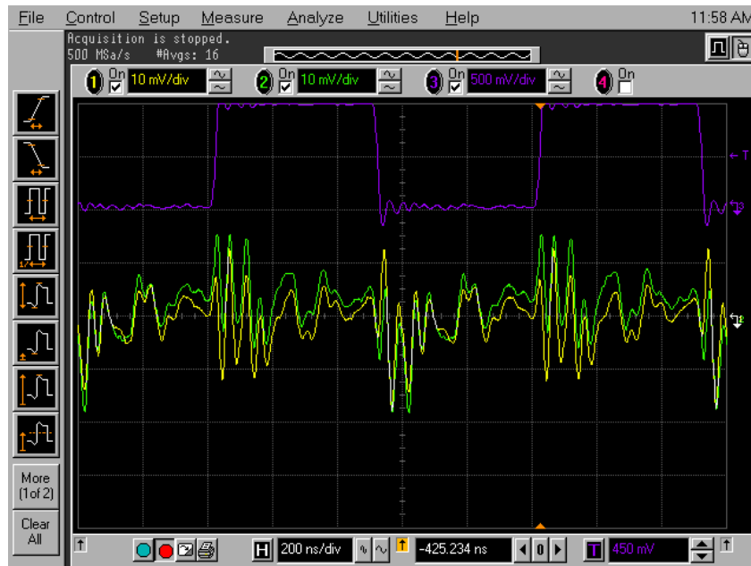
Figure 5-13: TIA Response to 10nA Input Current at 1MHz Clock Rate
