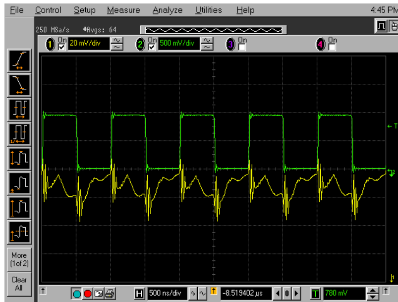
Figure 5-9: Response to a 100nA DC current at 1MHz clock
