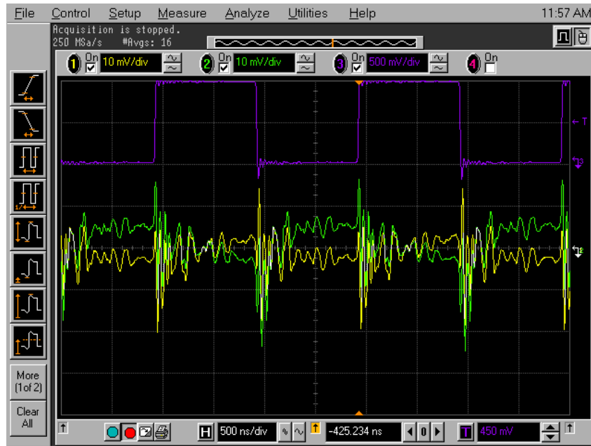
Figure 5-14: TIA Response to 10nA Input Current at 500 kHz Clock Rate
