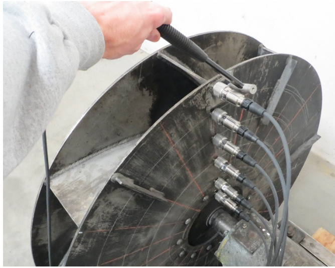
Figure 14. Accelerometers mounted with magnets and modal impact hammer.
