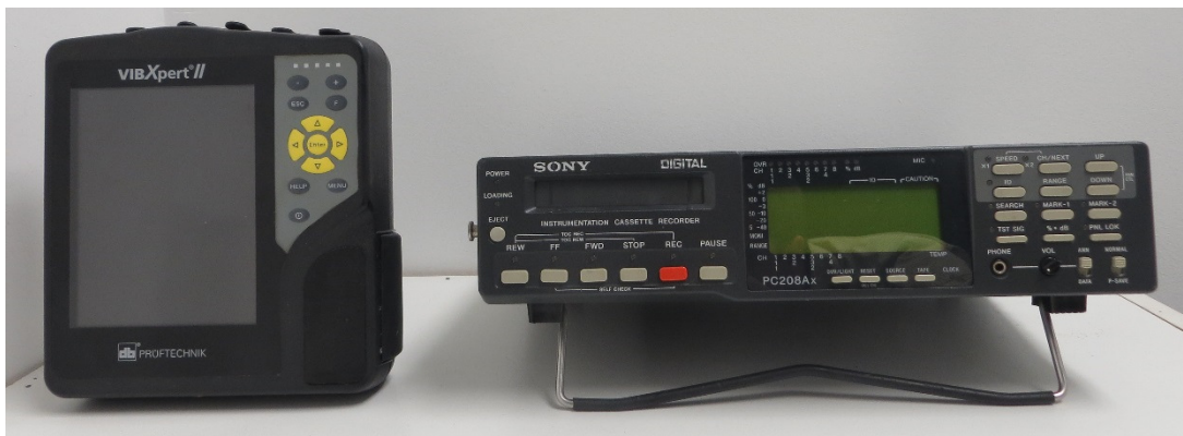
Figure 8. Portable 2-channel data collector and multi-channel recorder.
