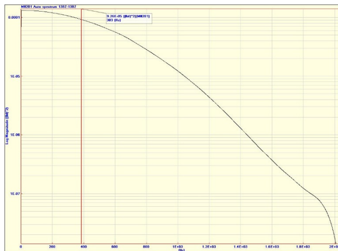
Figure 34. Auto spectrum of impulse showing the cut-off frequency as a red line.
