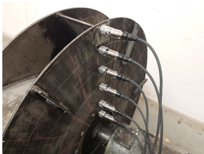
Figure 11. Placement of accelerometers on the fan back plate.
