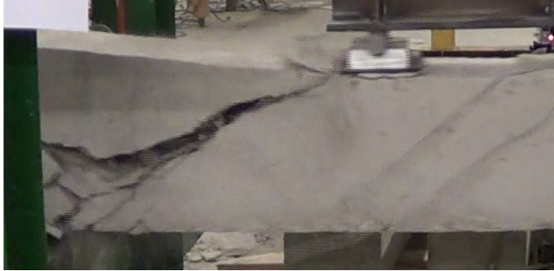
Figure 65: IIb-1 at time of collapse
