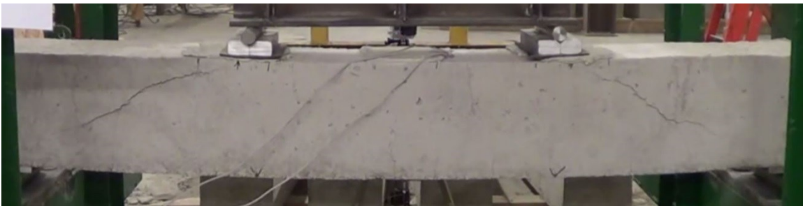
Figure 64: IIb-1 shear cracking before collapse event
