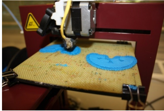
Figure 17: 3D printing in progress of type II form molds
