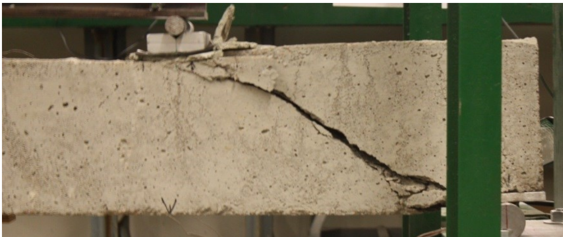
Figure 60: Ib-1 shear crack (rear view)
