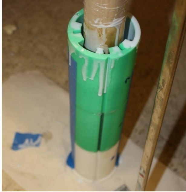
Figure 20: Type II silicone casting
