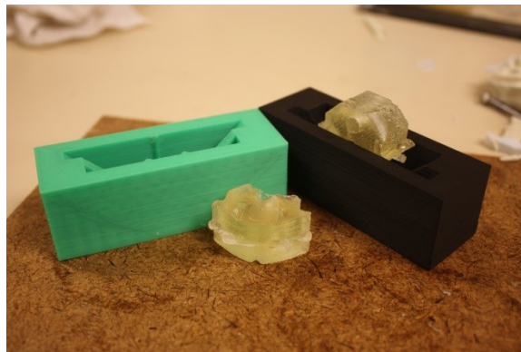
Figure 26: Type III form molds and support blocks
