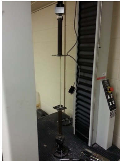
Figure 6: GFRP sample specimen in testing machine
