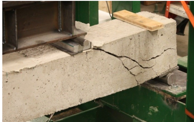
Figure 67: IIb-2 failure patterns before collapse
