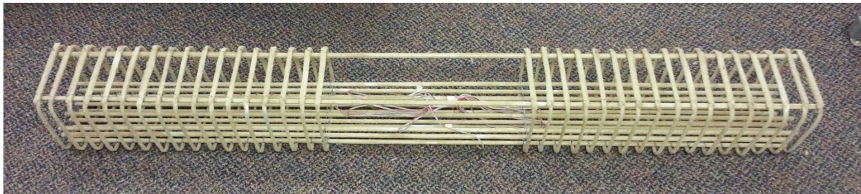
Figure 43: Type Ia reinforcement assembly
