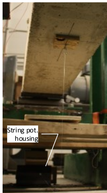
Figure 45: String potentiometer arrangement
