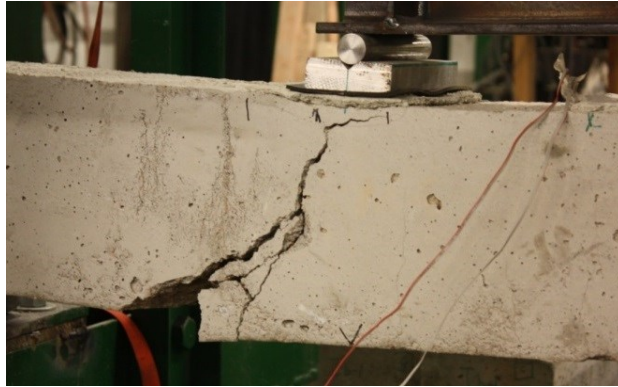
Figure 71: Type IIIb-2 specimen during loading
