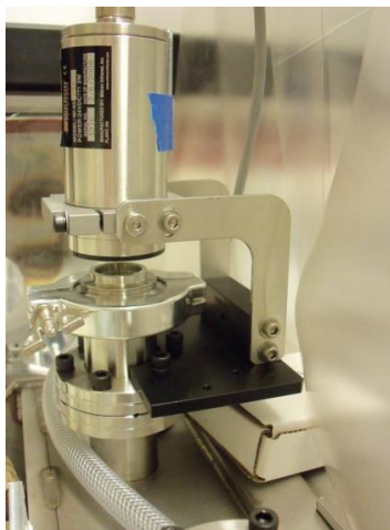
Figure 3-14: Mikron pyrometer installed on ARDS
