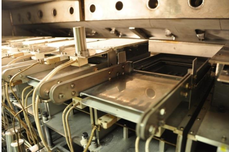
Figure 3-9: Heated pocket deposition source revealing pocket and shutter hardware
