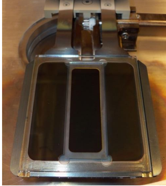
Figure 4-50: PGO ITO sample in quartz carrier post deposition
