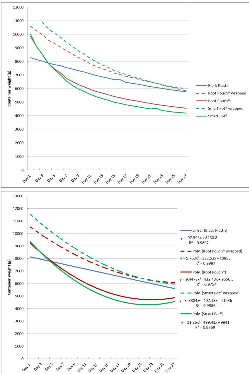
Figure 4.6. Water loss from black plastic (BP) and wrapped and unwrapped Root Pouch® and Smart Pot® containers during dry-down in the greenhouse (Experiment 2b). Regression lines shown in second figure.
