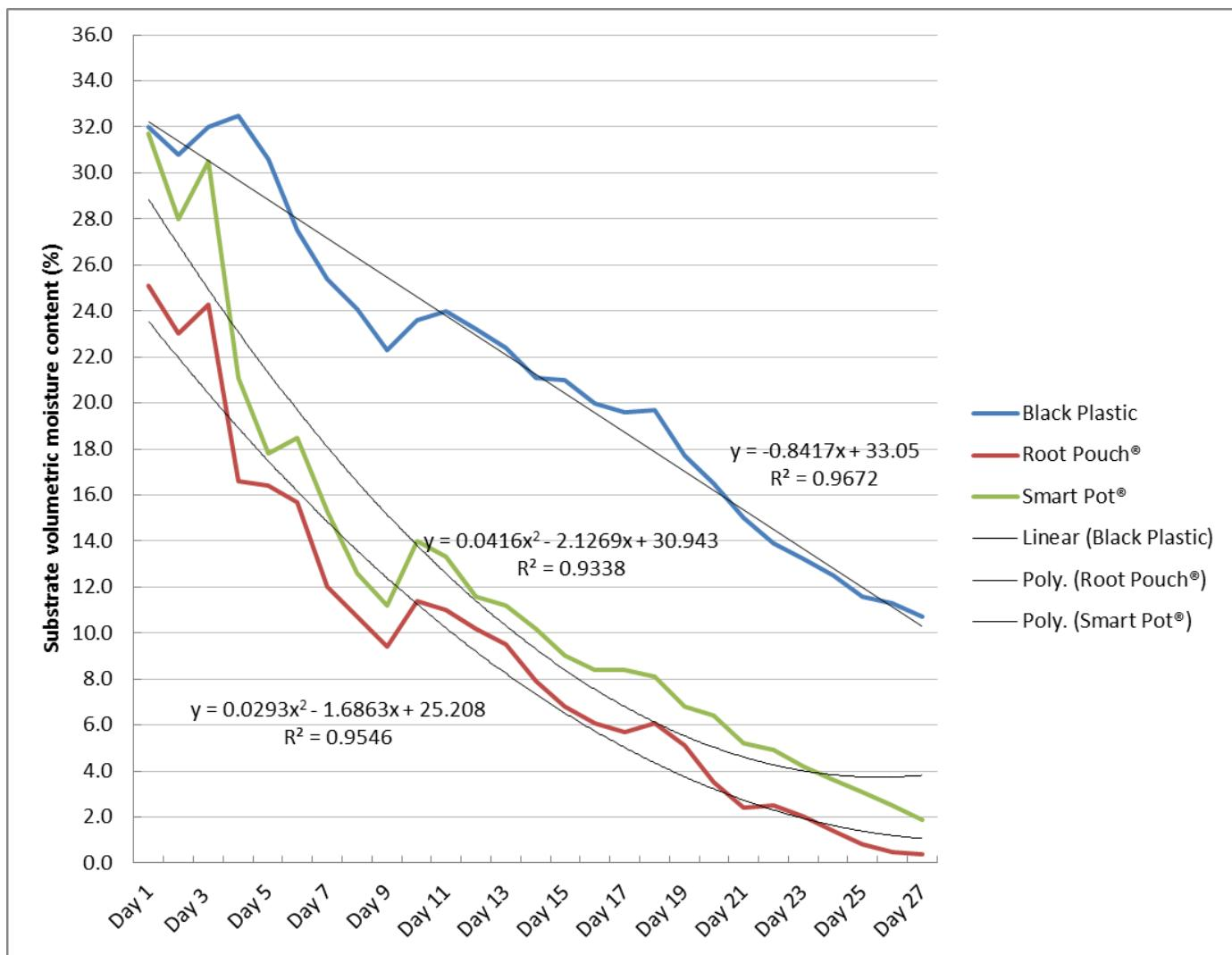
Figure 4.2. Substrate volumetric moisture content for black plastic (BP), Root Pouch® (RP) and Smart Pot® (SP) containers in the greenhouse (Experiment 1b).
