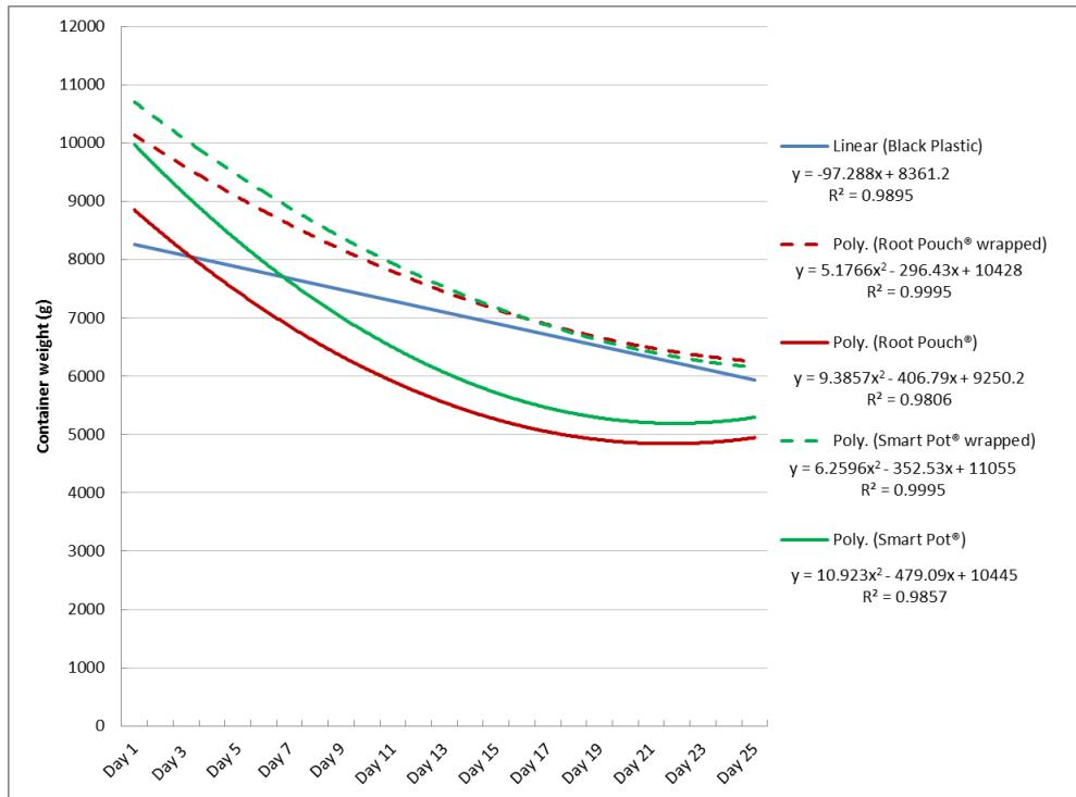
Figure 4.5. Water loss from black plastic (BP) and wrapped and unwrapped Root Pouch® and Smart Pot® containers during dry-down in the greenhouse (Experiment 2a). Regression lines shown in second figure.
