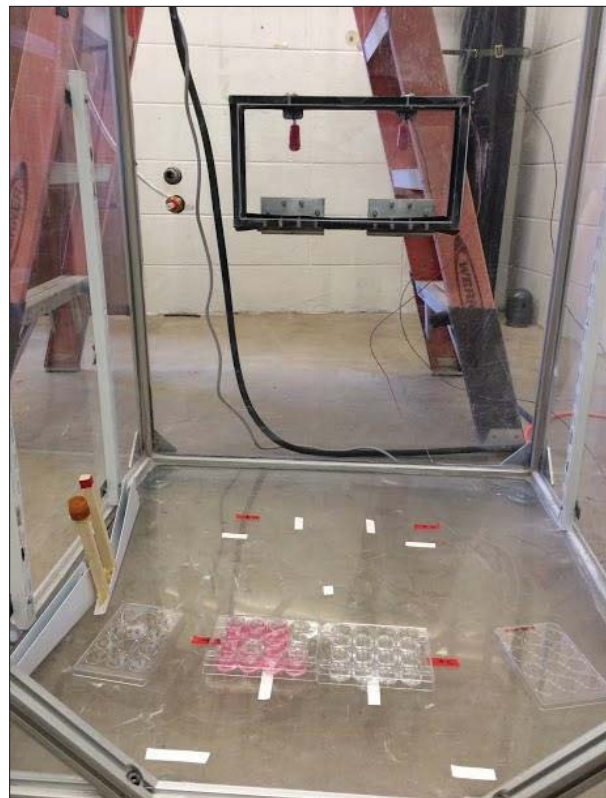
Figure 4-3. (A) Gravitational Settling Chamber used in PM_{>10} Cell Exposures (B) Cell Plate Placement during Ten Minute Settling Exposures. Dimensions: 1 m x 1 m x 2 m
