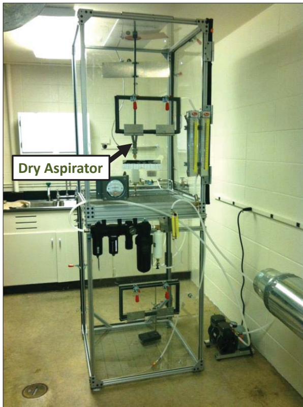
Figure 4-3. (A) Gravitational Settling Chamber used in PM_{>10} Cell Exposures (B) Cell Plate Placement during Ten Minute Settling Exposures. Dimensions: 1 m x 1 m x 2 m
