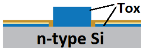
Figure 3.33: n-type thermal oxide chip cross section
