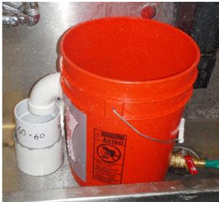
Figure 4-1: Basic flotation system used in this study
