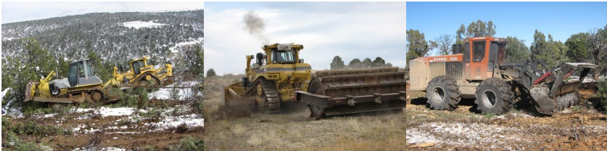
Figure 1.1. Heavy equipment used for pinyon-juniper removal. From left to right: anchor chain, rollerchopper, and mastication (or hydro-ax).
