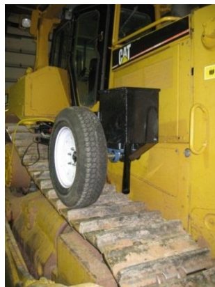
Figure 2.1. Seed dribbler mounted on bulldozer tracks. Species in seeding group 5 (Table 2.1) were seeded with the dribbler. Seeds were applied to half of each plot at two sites in northwest Colorado where pinyon-juniper canopy was removed using one of three mechanical treatments: anchor chain, rollerchopper, or hydro-ax (seed dribbler was used for chain and rollerchop treatments).
