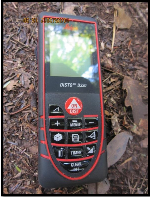
FIGURE 428: LASER DISTANCE METER USED FOR LEVEL II WIDTH MEASUREMENTS
