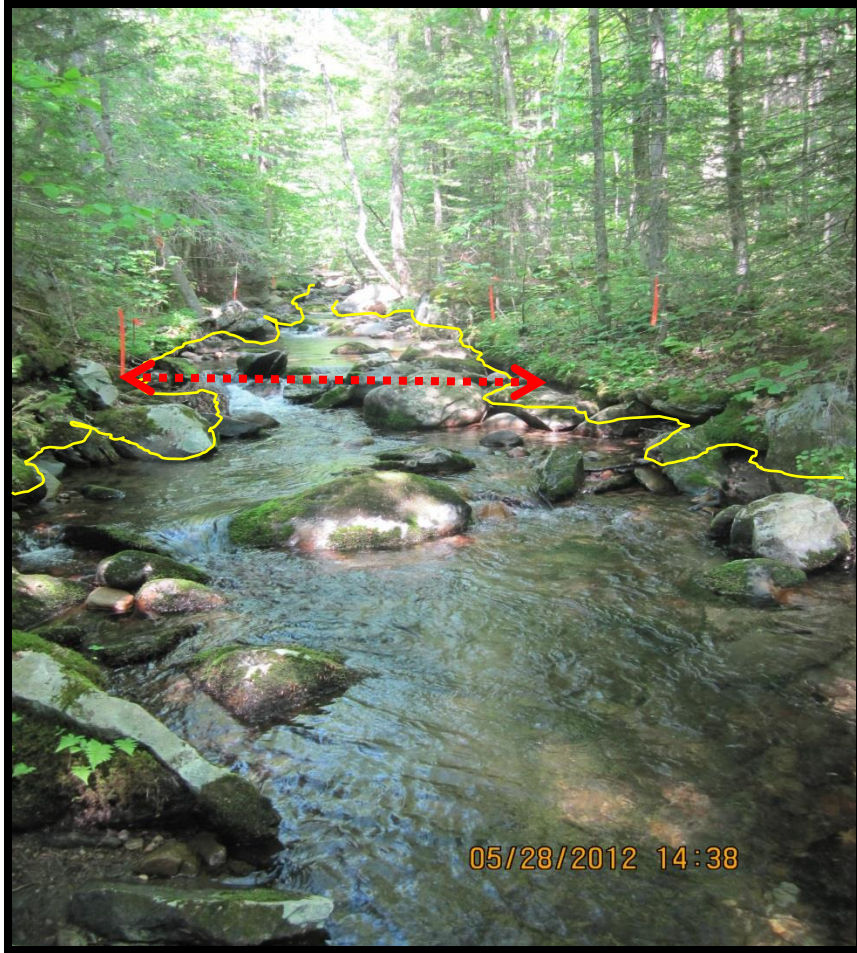
FIGURE 19: CATEGORIZING BANK IRREGULARITY BY THE LEVEL I PROTOCOL METHOD
