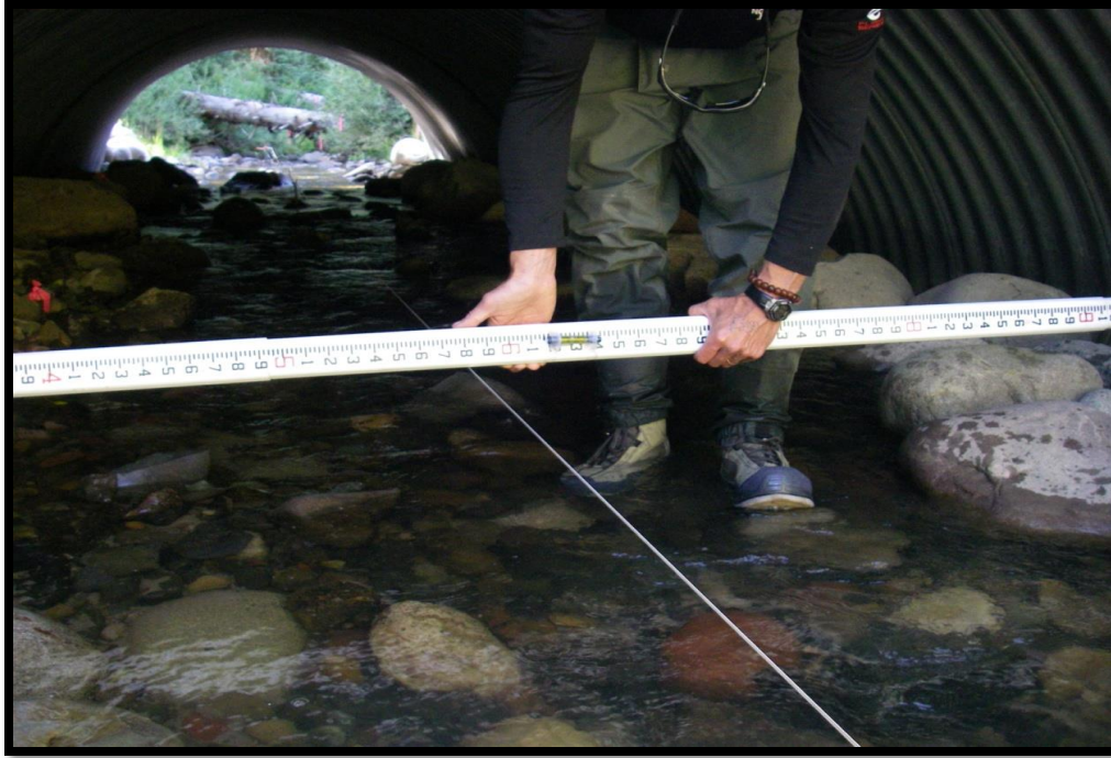
FIGURE 421: MEASURING WIDTHS WITH A LEVELED STADIA ROD AT THE HALF BANKFULL STAGE
