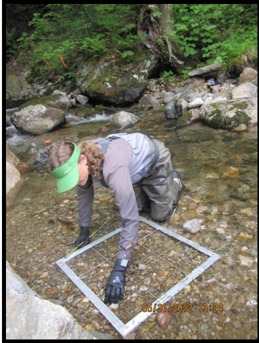
FIGURE 419: PEBBLE COUNT WITH THE ADJUSTABLE VERTICES SAMPLING FRAME
