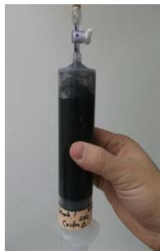
**Figure 4.4 Batch test with inoculated plastic media**
