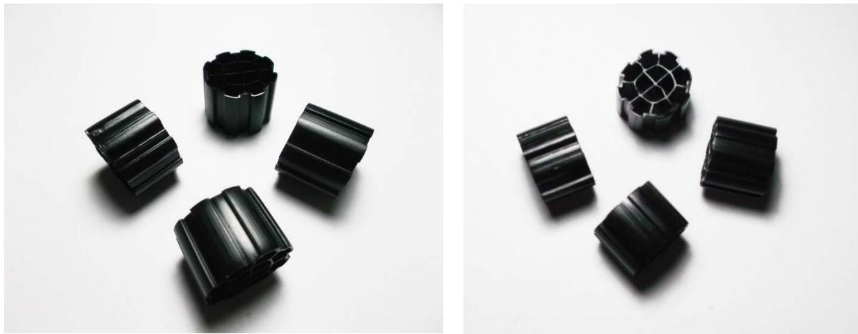
**Figure 4.2 Plastic media used in inoculation reactor**
