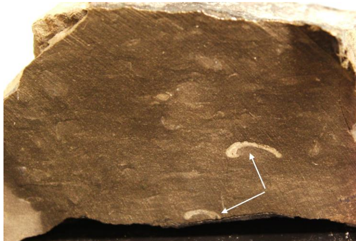
Figure 4.33: Sample K98_UBD; note the fossils (arrows) present in the sample. The sample is 6.7 cm wide by 4 cm tall.
