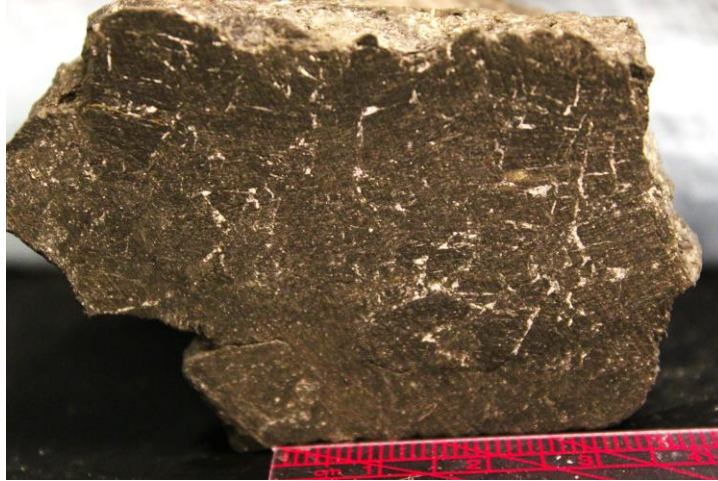
Figure 4.29: Sample K71+35; note the disrupted bedding and the abundant carbonate veins.
