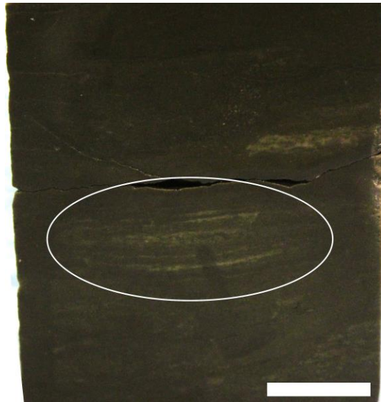
Figure 4.14: Sample K45+67. Note the lenses of lighter material (circled in white); these are not mineralization lenses. The white bar measures 1 cm.
