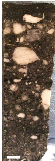
Figure 4.13: Sample K17-6; the top of the sample includes the bottom of the Kupferschiefer. Note the gradual decrease in grain size as depth increases. The white bar measures 1 cm.
