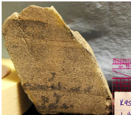
Figure 4.34: Sample K95-120; note the banded sulfide mineralization, with blebs branching off from the bands.
