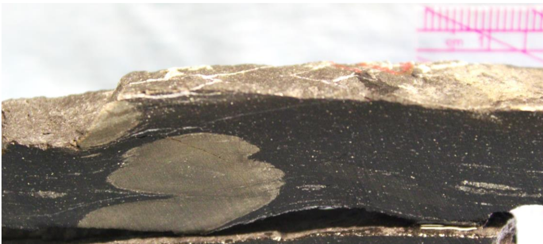
Figure 4.26: Sample K62+50; note the alternating lenses and the carbonate pods.
