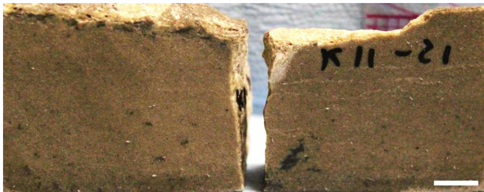
Figure 4.8: Sample K11-21; note the discontinuous fractures associated with whiter sand grains in the right half of the sample. The white bar measures 1 cm.
