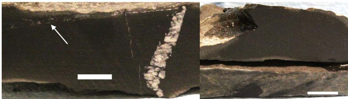
Figure 4.5: Left: Sample K2+26; note the thick carbonate vein and the thinner vein to the left. The white arrow points to the vein that appears to wander in and out of the cross section. Right: Sample K3+24; note the difference between the black, carbonaceous piece and the gray, carbonate face of the lower piece. The white bars measure 1 cm.
