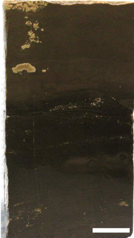
Figure 4.16: Sample K42+33; note the color change two thirds of the way up the sample. The white bar measures 1 cm.
