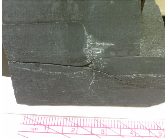
Figure 5.2: Sample K53+20 from core E-27; note the bedding-perpendicular vein with bedding-parallel spreading. Note that the photomicrograph was taken while the sample was dry.
