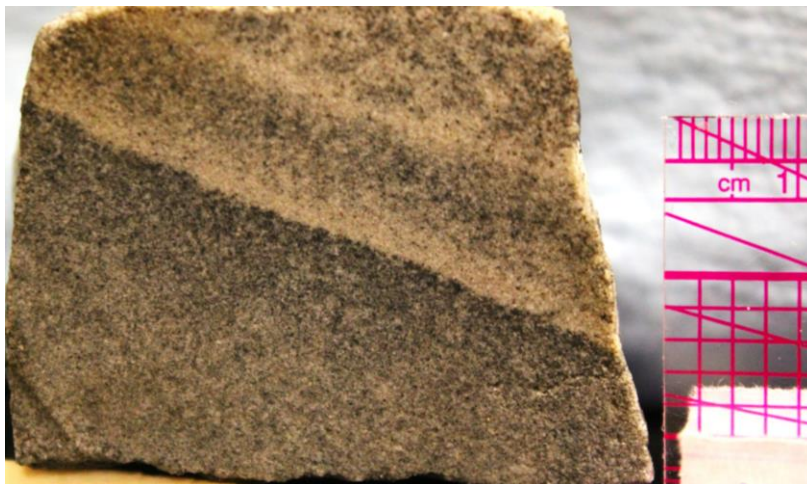
Figure 4.31: Sample K94-120; note the bands of sulfide mineralization, and the two types of contact: sharp and gradational.
