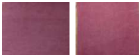
Figure 14. Fabrics printed with Vat Red 13 using Proso millet starch (left) and sodium alginate (right)
