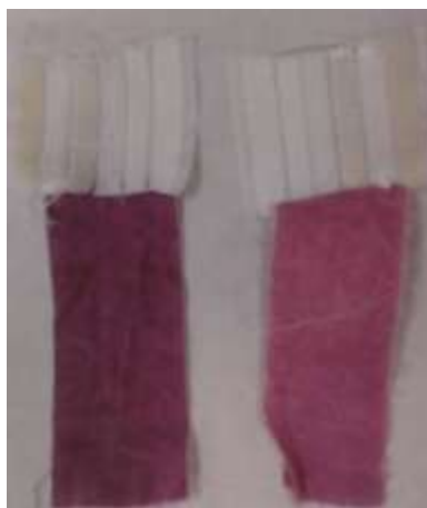
Figure 23. Washing fastness of fabrics printed with Vat Red 13 using Sorghum starch (left) and sodium alginate (right)
