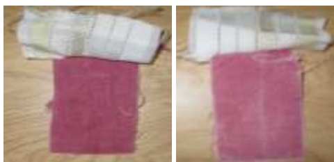
Figure 15. Washing fastness of fabrics printed with Vat Red 13 using proso millet starch (left) and sodium alginate (right)
