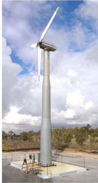
Figure 2-2: Experimental Setup at UCSD (I Prowell et al., 2008)
