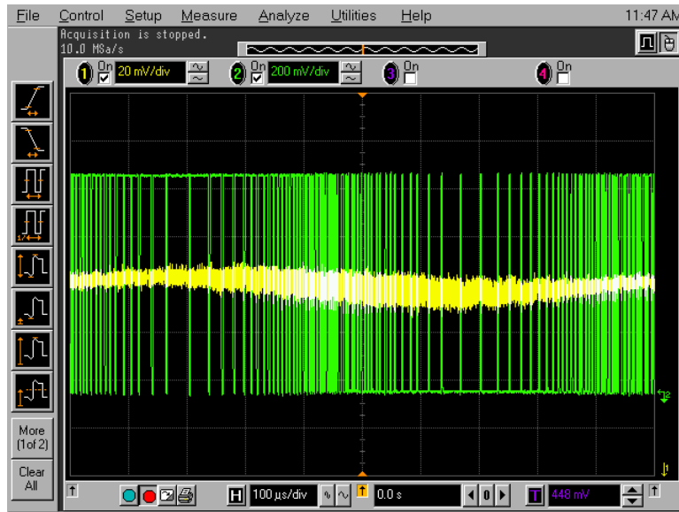
Figure 5-19: Main-amplifier and 2 nd order modulator signal chain with 1MHz clock
