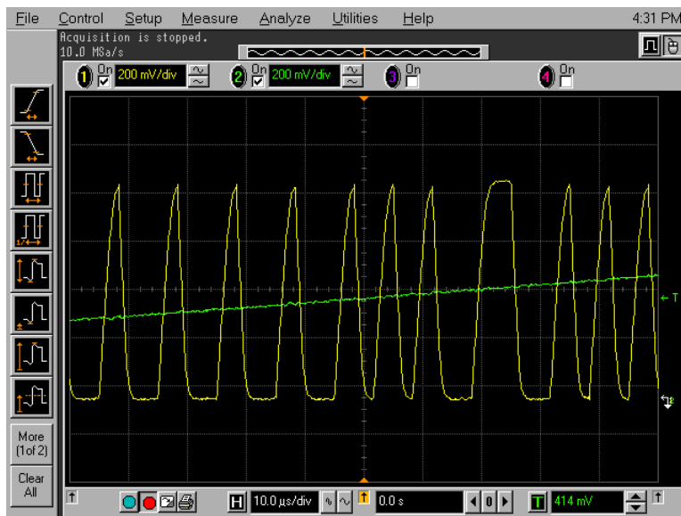
Figure 5-13: Modulator output with 300 kHz clock
