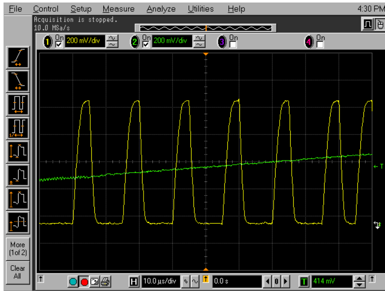
Figure 5-12: Modulator output with 200 kHz clock
