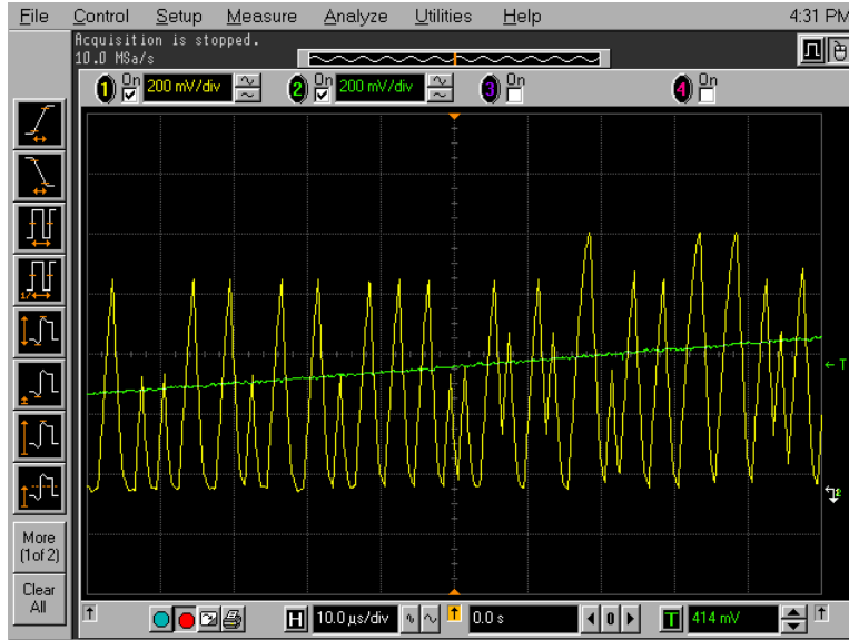
Figure 5-14: Modulator output with 1 MHz clock
