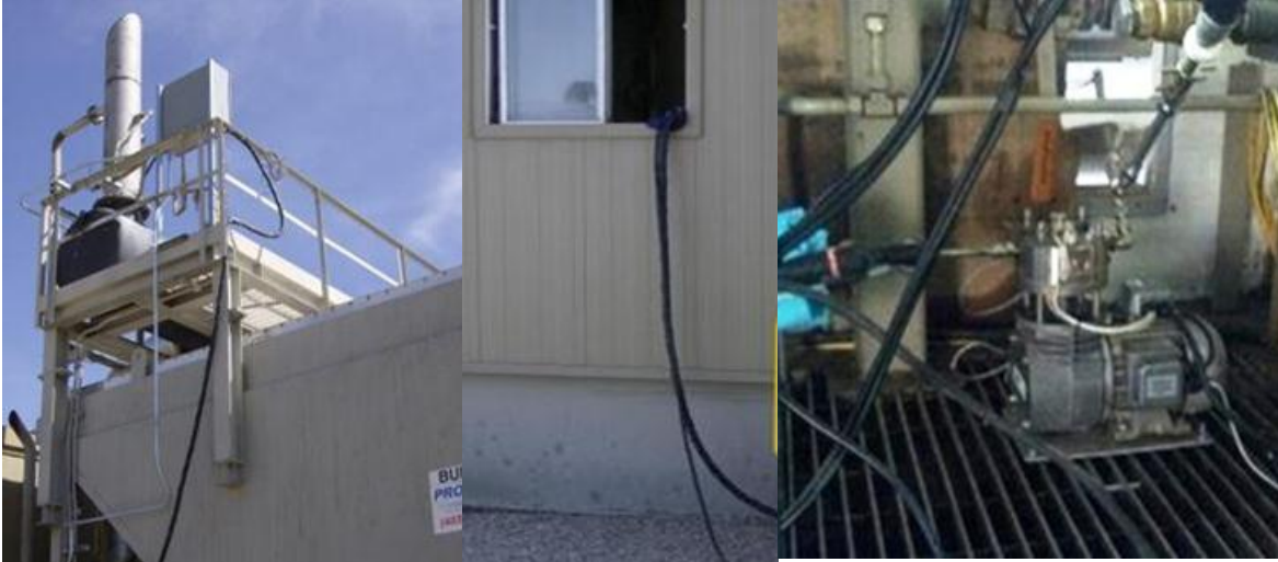
Figure 17: Heated sample line is routed from the sampling port on the elevated catwalk (left), through a ground level window in the engine room (middle), to the inlet of the heated head pump (right).
