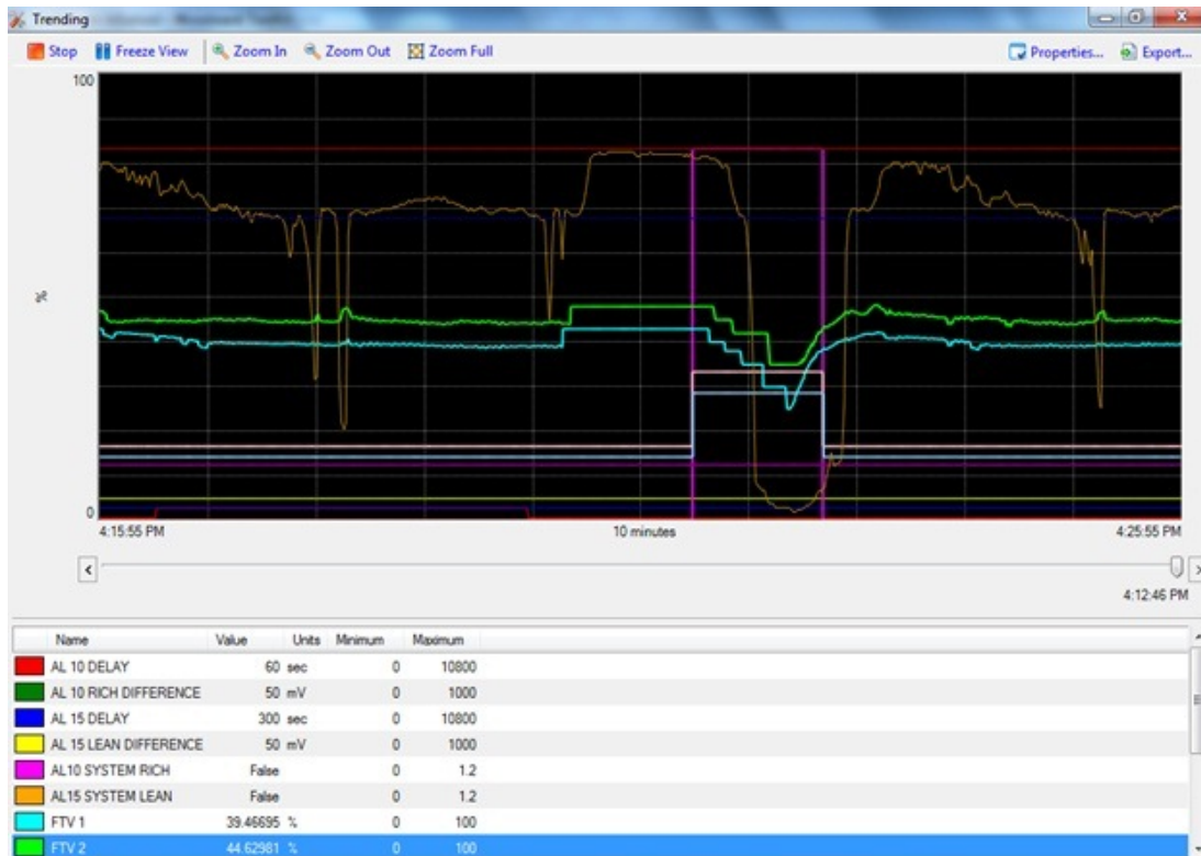
Figure 63: E3RB ToolKit trends displaying alarms for System Lean (orange trend - above) and System Rich (magenta trend - below) conditions.
