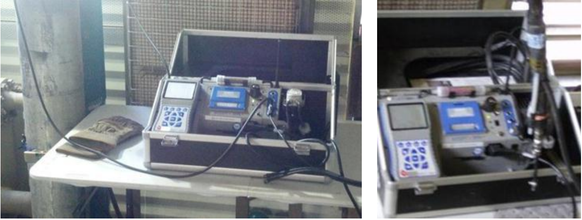
Figure 18: (Left) Portable emissions analyzer setup inside the engine room. (Right) Alternate arrangement for exhaust sampling: heated sample line (hanging in foreground) ready for direct connection to the sampling port on the analyzer.
