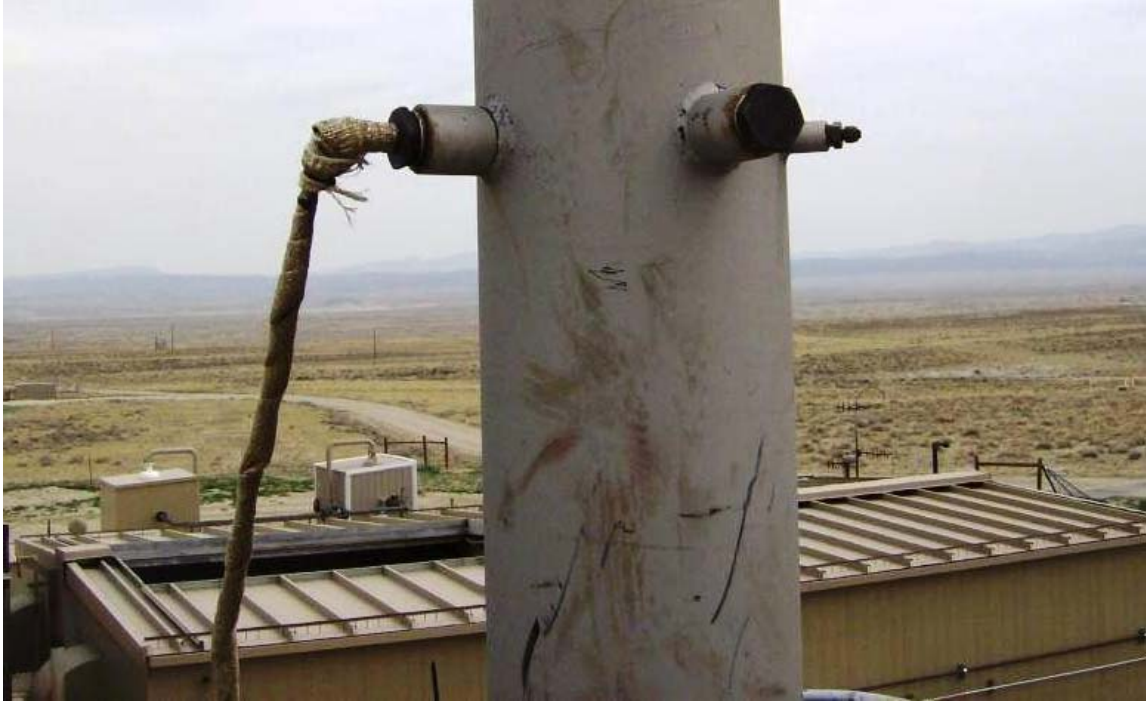
Figure 15: Post-catalyst emissions sampling probe in exhaust manifold.
