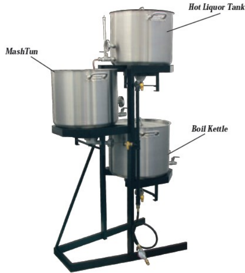
Figure 3.1 Brewing system used to produce beers
