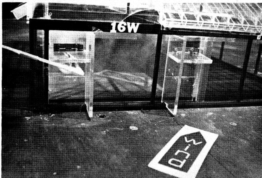
Figure 7-5-2. Flow Visualization for Configuration IV of the PCL with Wing Walls
