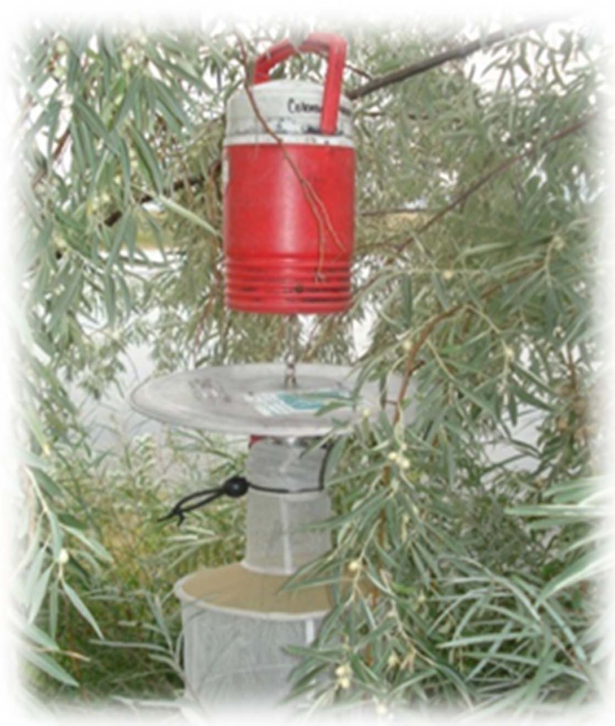
Figure 3.2 CDC CO 2 baited light traps used in the collection of adult Cx. tarsalis mosquitoes. Photo obtained from Colorado Mosquito Control, Inc.
