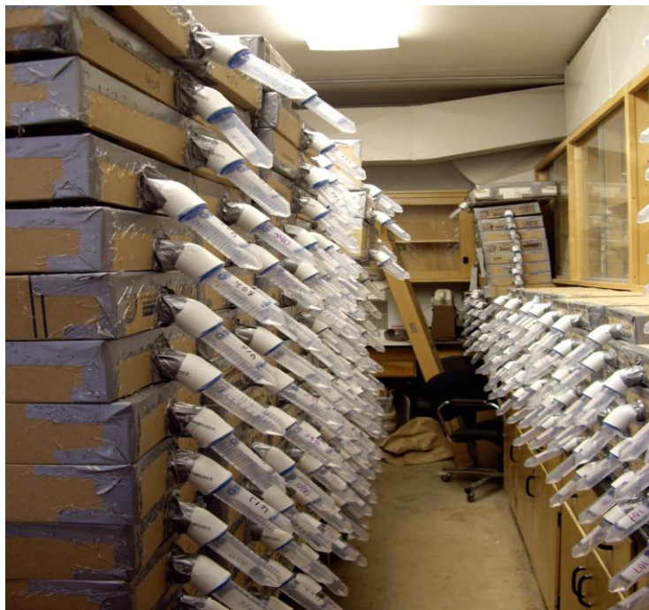
Figure 2.4 Emergence containers constructed from cardboard boxes and adapted with 50 mL collection tubes.
