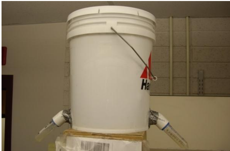
Figure 1.1 Adult choice test. Walnut twig beetle infested log was placed inside of bucket and beetle emergence into the two tubs was recorded. Tubes were filled with either \frac{1}{4} -strength potato dextrose agar modified with 100mg/liter streptomycin sulfate and 100mg/liter chloramphenicol (PDA) or PDA colonized by G. morbida .
