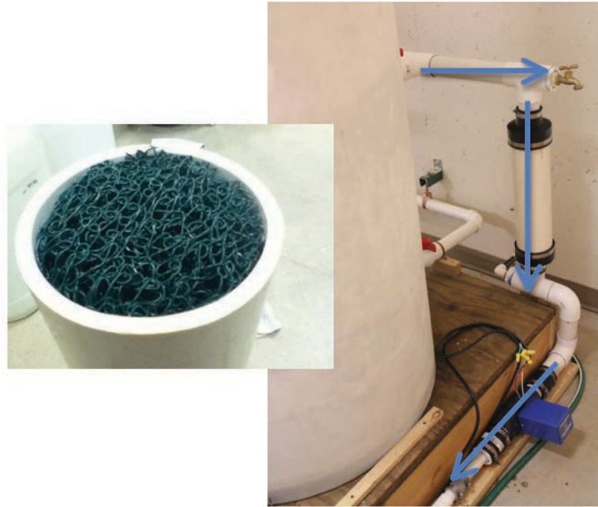
Figure 3.5 Coarse Matala Filter
