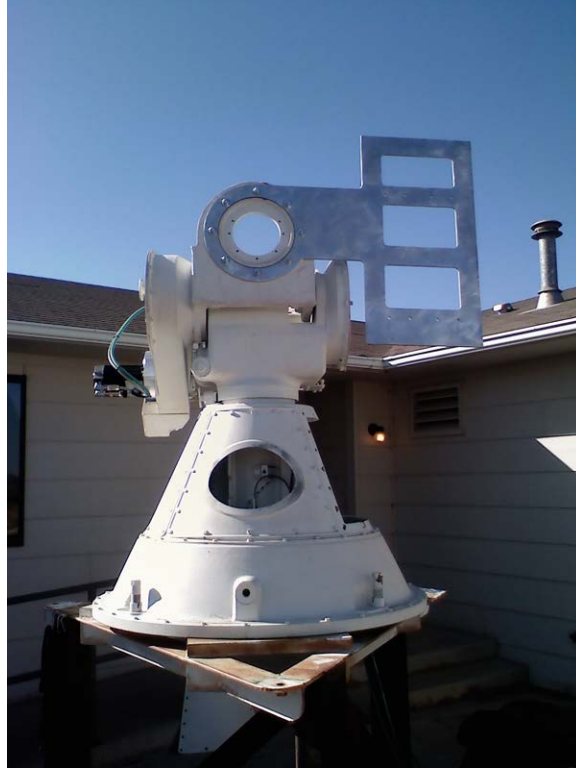
Figure 2.4: SCR-584 pedestal with EL motor and Transceiver mounting plate, shown without antenna and mounted on work stand
