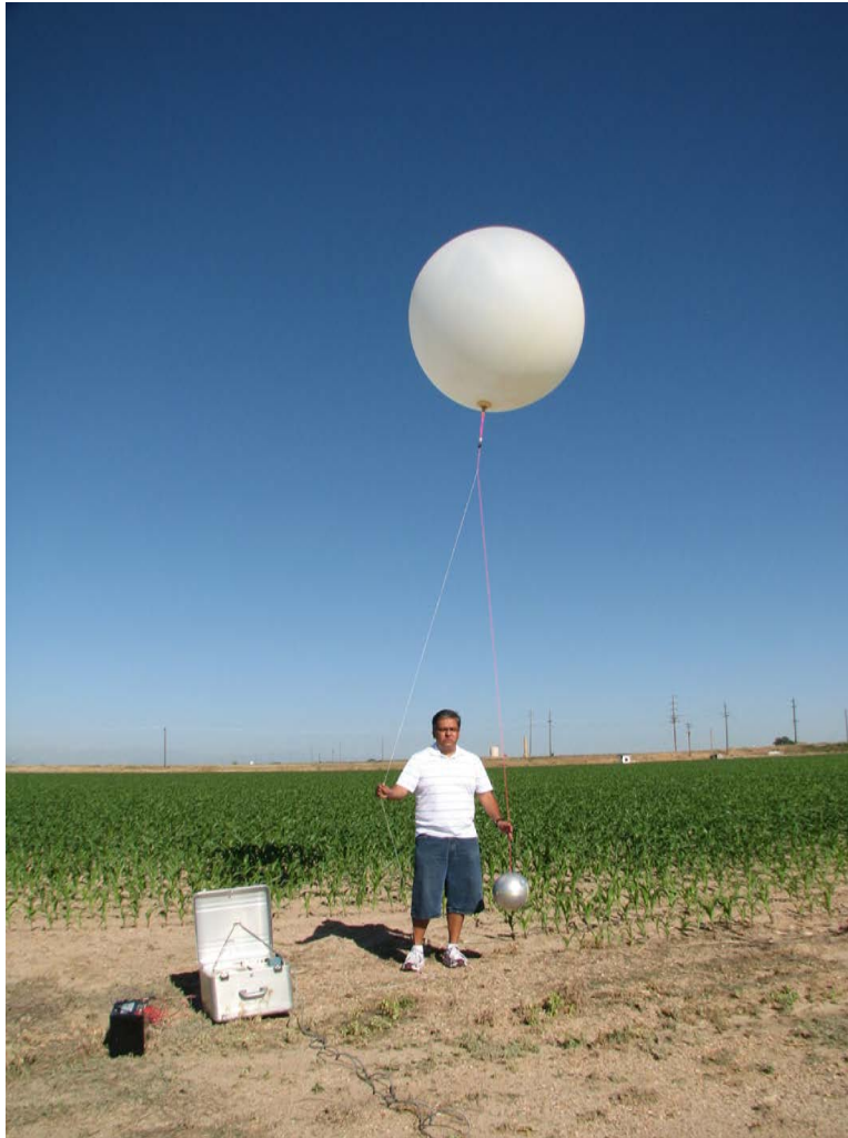
Figure 2.12: Launching balloon and tethered metal sphere using electric winch
