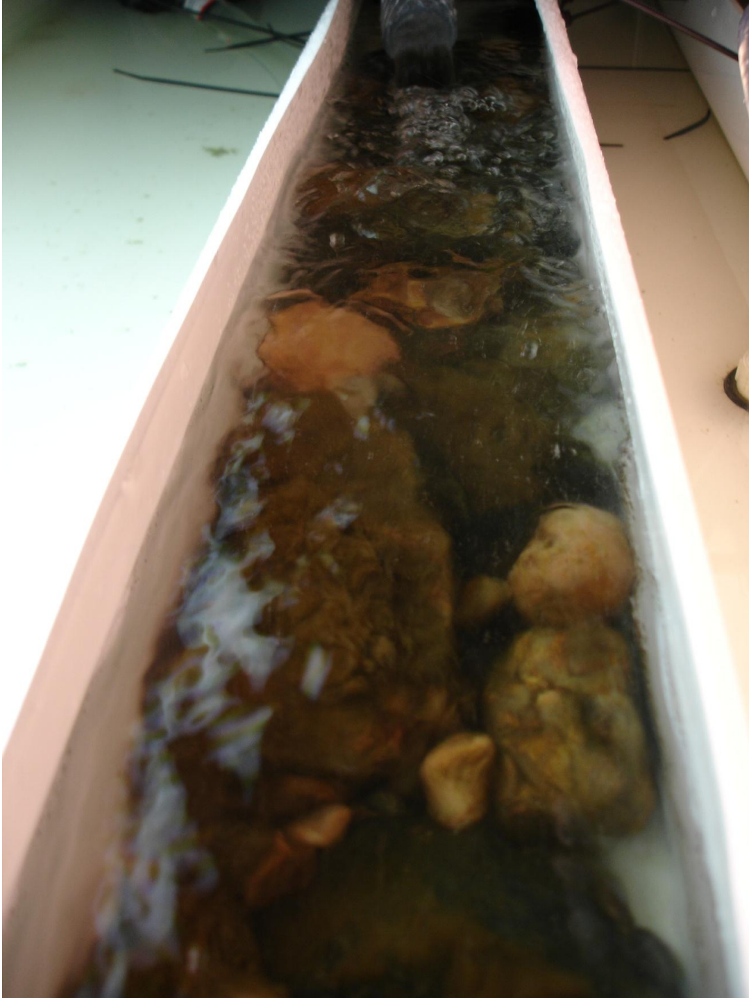
Figure C.4 - Close up of deep trough setup looking downstream. Rocks colonized by Didymo can be seen.
