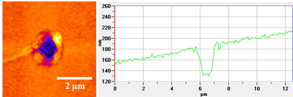
Figure 4-15. AFM micrograph of a CGH reconstructed in PMMA with a lineout showing the ablation crater below.
