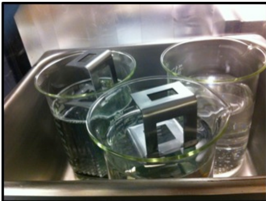
Figure 4. 31: Substrates cleaning setup inside the ultrasonic washing machine within the mini-environment.
