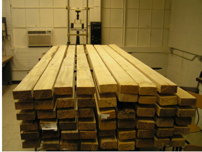
Figure 8. Two by Fours stickered in temperature and humidity controlled room. 22
