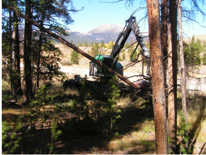
Figure 7. Harvester cutting and delimiting a tree 19
