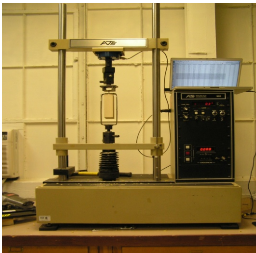
Figure 10. ATS Apparatus withdrawing nail from cross section of block 30
