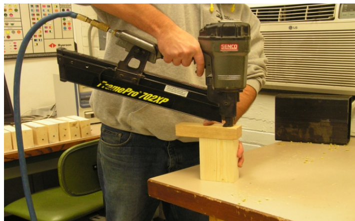
Figure 11. Pneumatic nailing procedure utilizing spacer block to seat nail in cross section of block 32
