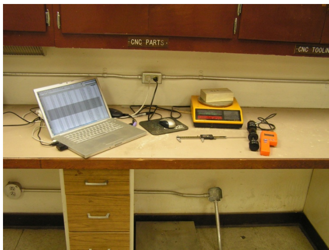
Figure 9. Workstation used to determine moisture content and specific gravity of each block, including calipers, scale, and moisture content reader 26
