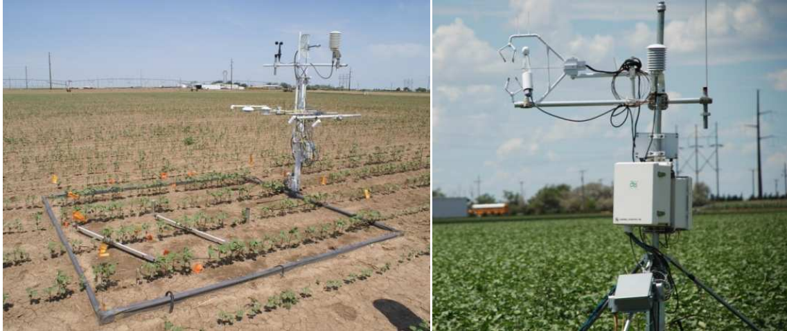
Figure 3.1: Lysimeter box with micrometeorological instrumentation (a) and eddy covariance system (b). Photographs courtesy of José Luis Chávez.
