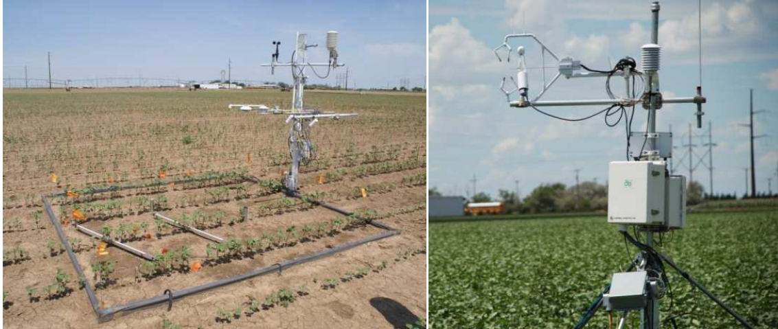
Figure 2.1: Lysimeter box with micrometeorological instrumentation (a) and eddy covariance system (b). Photographs courtesy of José Luis Chávez.
