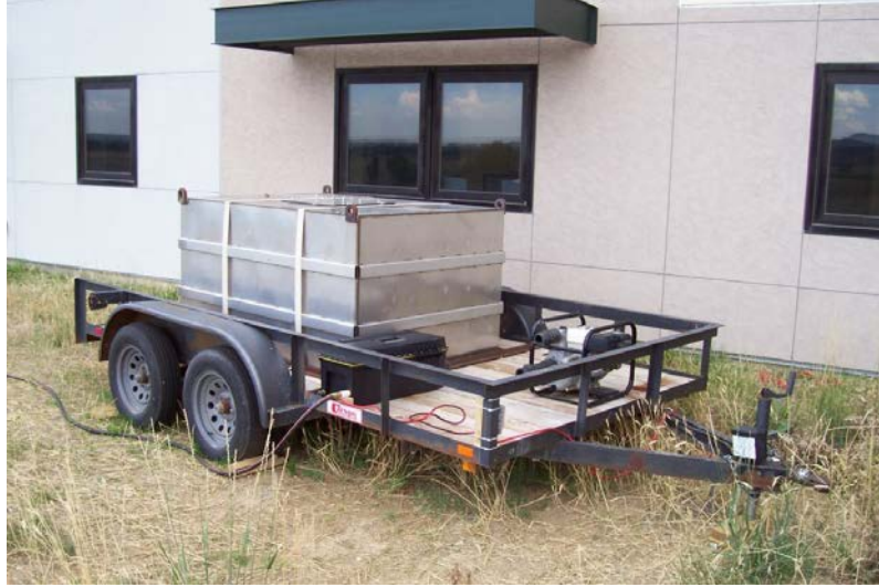
Figure 4.5. 500 Gallon Trailor used to Transport Graywater from the Residence Halls to the Wetlands.
