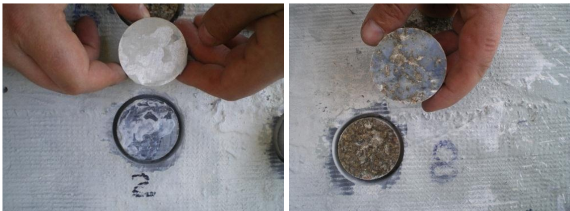
Figure 3.40 and 3.41. Failure Mode A: bonding adhesive failure at loading fixture (on left), Failure Mode E: Adhesive failure at CFRP/substrate adhesive interface (on right)
