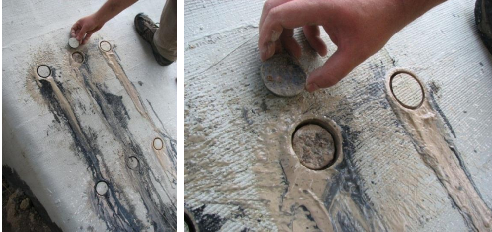
Figures 3.27 and 3.28. The core drilling location that failed due to torsional stresses during the core drilling process, bay 1NW
