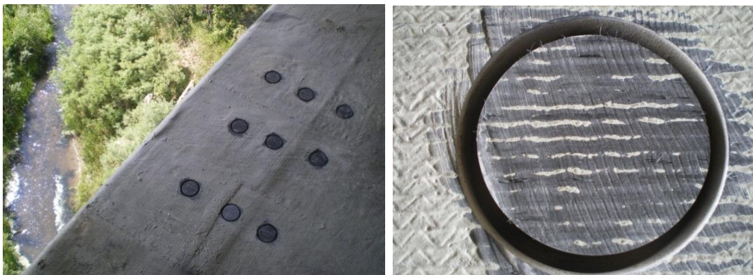
Figures 3.31 and 3.32. Prepared areas for the adhesion of aluminum pucks for pull-off tests and a close-up of a prepared surface
